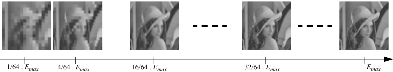
Fig. 8. Illustrating the incremental refinement property with respect to computational energy of the FM-IDCT algorithm
