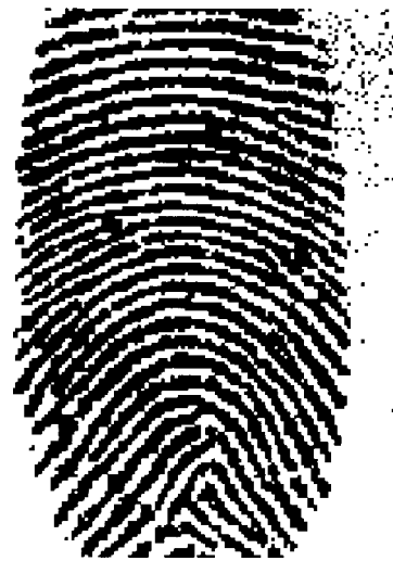
Fig. 11. Binarized fingerprint image from sensing circuits without any additional signal processing.
