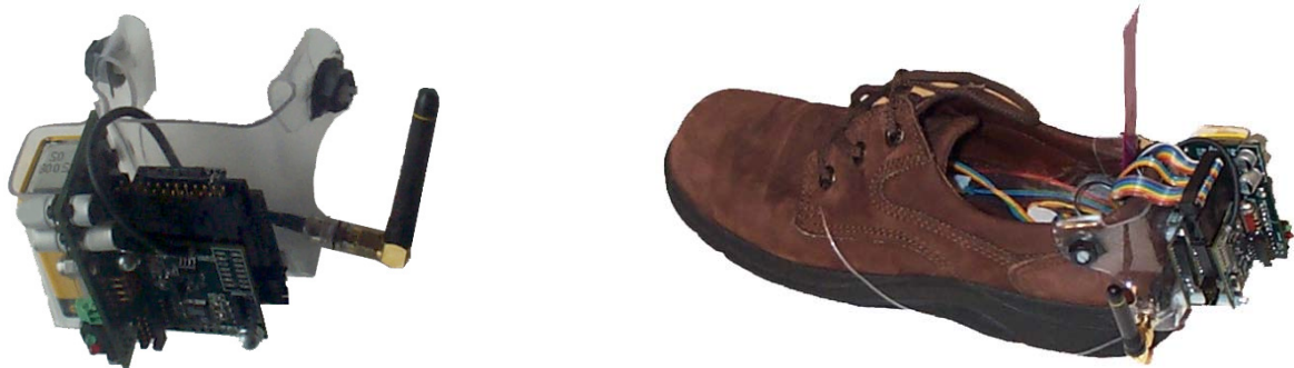
Figure 2: The sensor stack alone, and mounted on a shoe.
