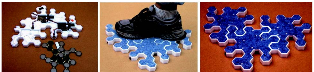
Fig 11 Prototype Z-tiles hardware — (left) showing FSR sensors and processing electronics, and (centre/right) snapped together to form a sensor network.
