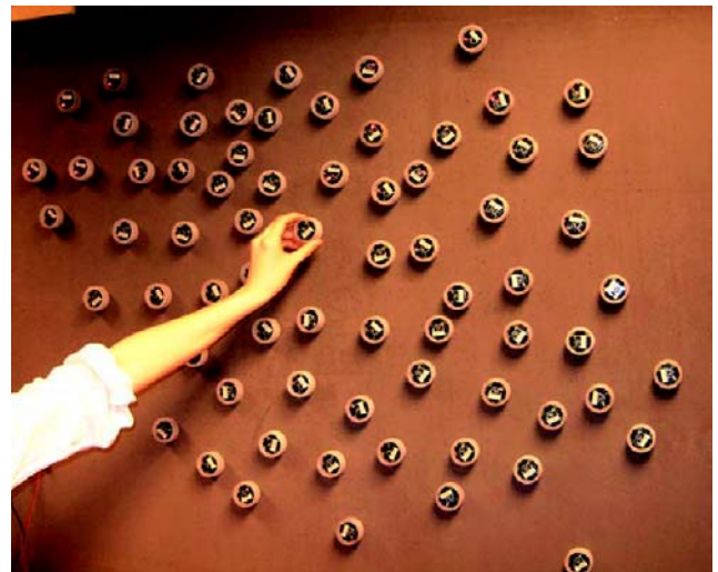
Fig 2 The Pushpin computer and its power plane.
