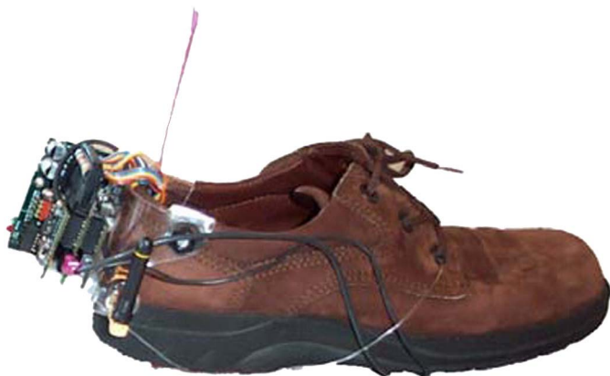
Fig. 3. Wearable Gait Analysis Platform (sensors on heel)
