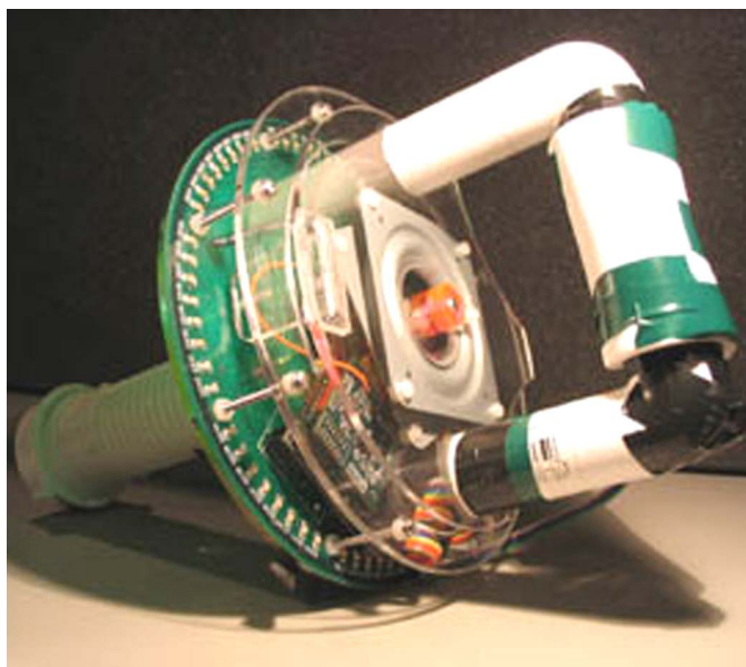
Fig. 4. FlexiGesture Controller (sensors between plexiglass and large PCB)
