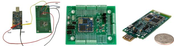
**Figure 4. (a) An illustration of how simple iCount is to implement: a Maxim MAX1724 switcher is connected to a Moteiv Tmote. (b) A sensor node for environmental monitoring includes iCount support which allows expected energy usage to be compared with actual energy usage. (c) A testbed node for benchmarking applications includes iCount plus five decades of precision calibration circuitry.**
