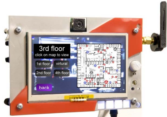
Figure 1. A Ubiquitous Sensor Portal (USP)
