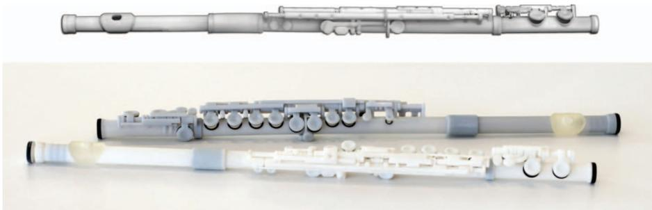
Fig. 1. Pictures of the printed flutes—FDM technology—made from acrylonitrile butadiene styrene (ABS) (top), and PolyJet technology—two flutes, each made from three different materials (bottom).
