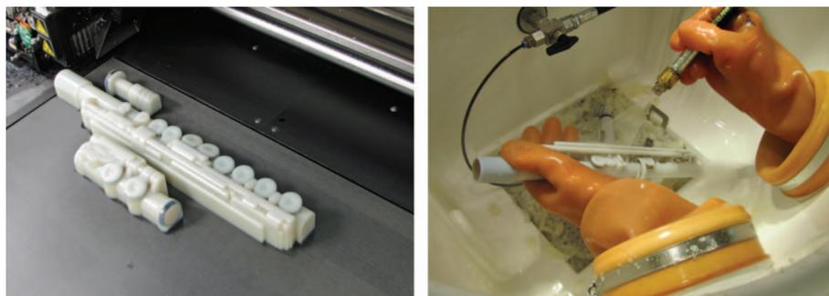
Fig. 2. Printed flute parts by Objet Connex500, covered with support material (left), and the cleaning process (right).
