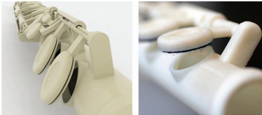
Fig. 4. The design of the printed plastic pads (left), and a picture of the glued felt solution (right) for the FDM flute. The computer rendering in the left was made using V-Ray software.
