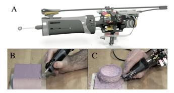
Figure 1: (A) The FreeD and (B-C) the process of making a bowl from polyethylene foam.
