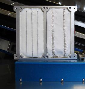
further. Our collaborators in the Fibers@MIT group, for example, use a manufacturing technique called thermal drawing, in which a centimeter-thick sandwich of materials is heated and stretched to submillimeter thickness, like pulling a multicolored taffy. Incredibly, the internal structure of the resulting fiber remains highly precise, yielding functional devices such as sensors for vibration, light, and temperature that can be woven directly into fabrics.
