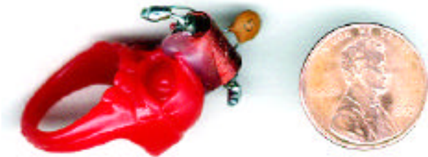
Figure 2: Small LC tag mounted on child's plastic ring
