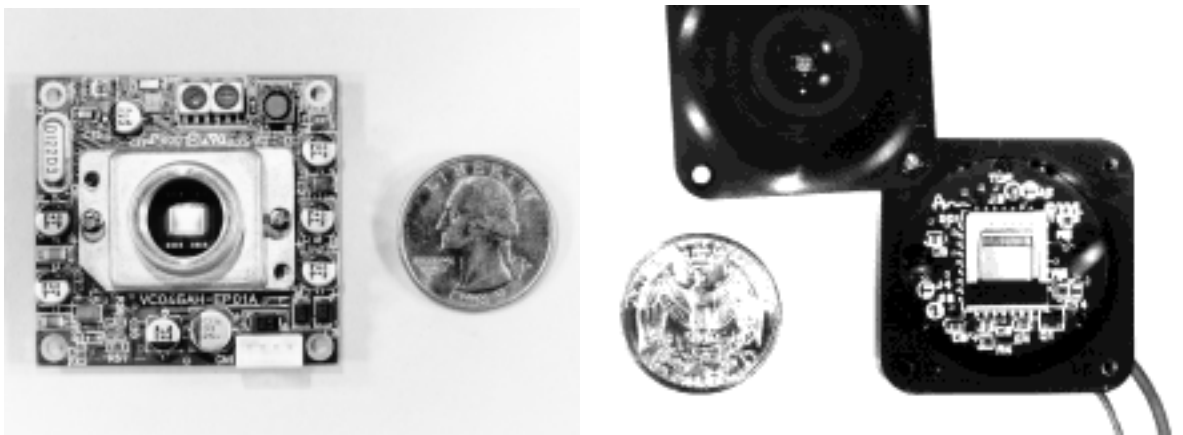
Figure 4: Miniature monochrome cameras for VSM application from Chinon (left) and VVL (right)
