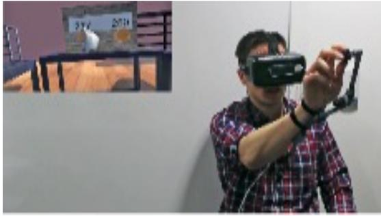
Figure 7: FeelIO - Wearable robot arm with a knob [46]
