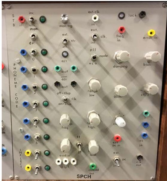
**Figure 11: The Phoneme Generator module, with XOR'ed switches and input bits at left**
