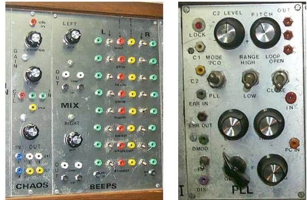
**Figure 10: The Voltage-Controlled Chaos and Alarms Modules (left) and a Phase-Locked Loop (Right)**
