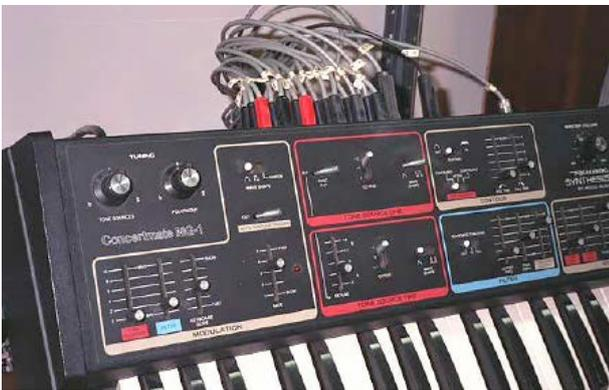
Figure 13: Umbilical cables connecting to customized patchpoints at the rear of the MG-1. The other end of this cable runs to an Interface module analogous to that above
