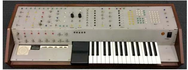
Figure 15: The Assimilated VL-Tone (the original device is embedded at lower left)
