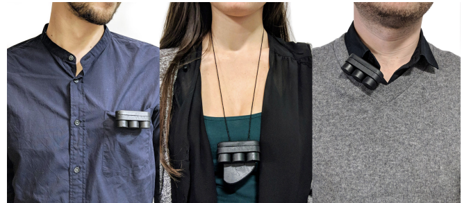
Fig. 1. BioEssence is a wearable olfactory display that can be worn as a clip or as a necklace. The device can easily be attached to pockets, shirt necklines, jewelry threads, and cords.
