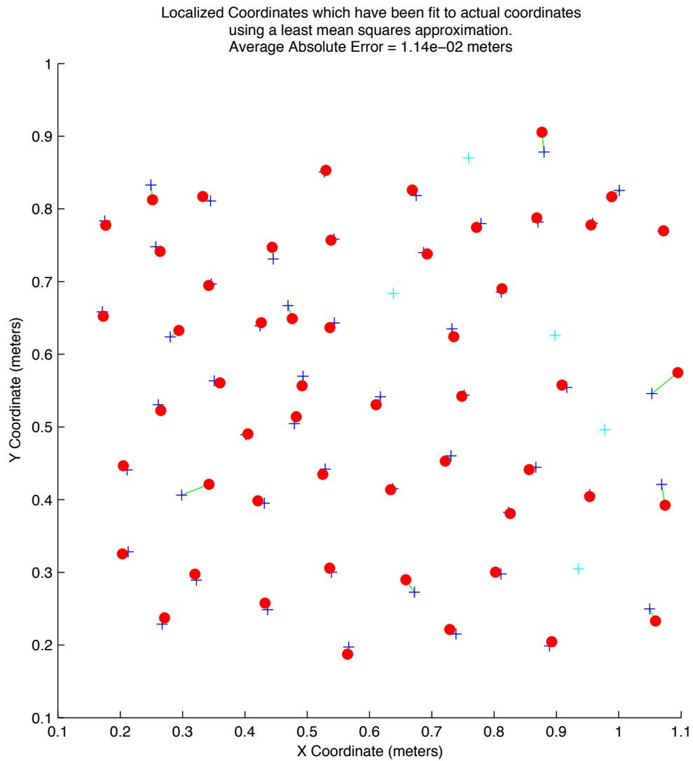
Figure 5-6: Estimated Pushpin coordinates generated using the SGD/MR system that have been aligned with measured coordinates via a LLSE fit. The crosses denote measured coordinates and the circles denote coordinates estimated using lateration. The line connecting each cross to a circle indicates which estimated coordinate corresponds to which measured coordinate. Cyan colored nodes have been rejected as outliers.
