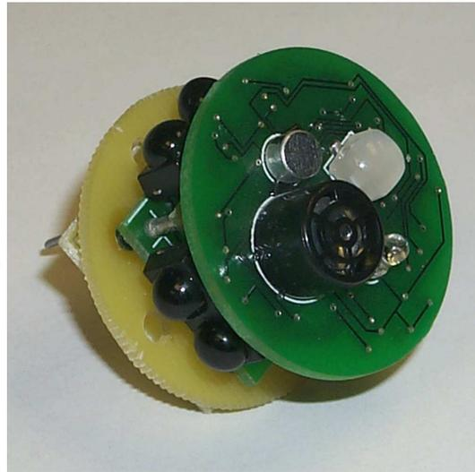
Figure 2-6: A pushpin with the Time of Flight (TOF) Expansion module shown attached to a Pushpin. The TOF module contains an RGB LED, microphone, photo-transistor, and sonar transducer. The last two of these are used to measure sonar time of flight for use in localization.
