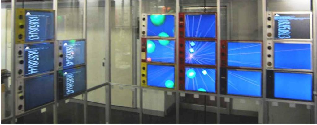
Figure 3-1: Smart Architectural Surfaces tiles mounted on a frame along two glass walls. A distributed data display can be seen across the screens of one wall. This picture is excerpted from Dalton's thesis [15].
