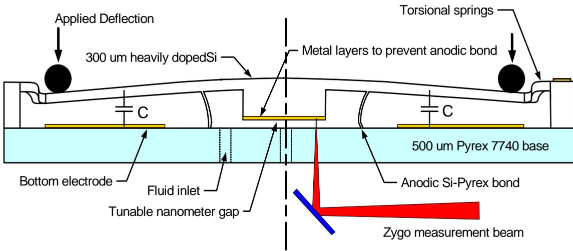
**Figure 1: Cross section of the Nanogate with Added Capacitive Sensor Electrodes**
