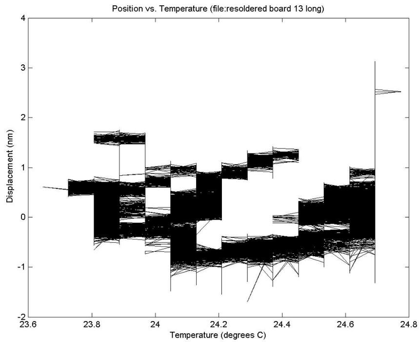
**Figure 32: Temperature dependence of drift**
