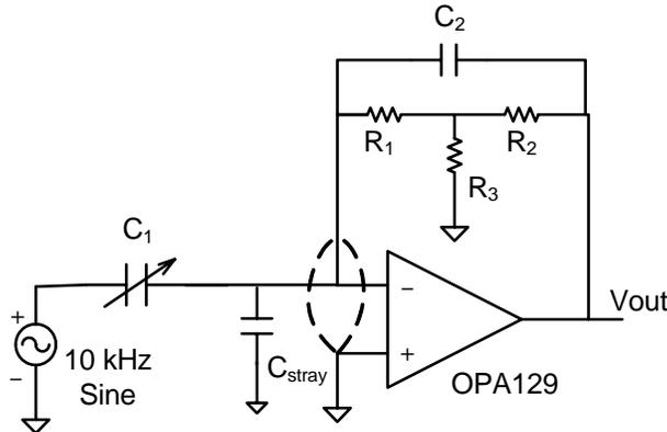
**Figure 14: Input Amplifier Schematic**
