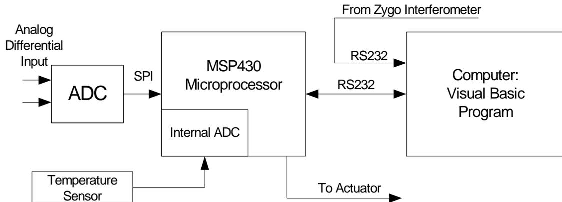
**Figure 17: Data Acquisition System**
