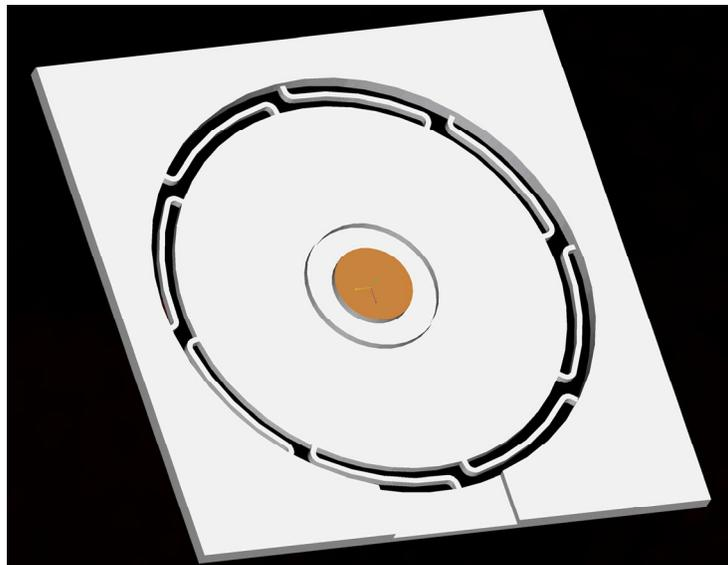
**Figure 2: CAD model of the Nanogate silicon diaphragm**
