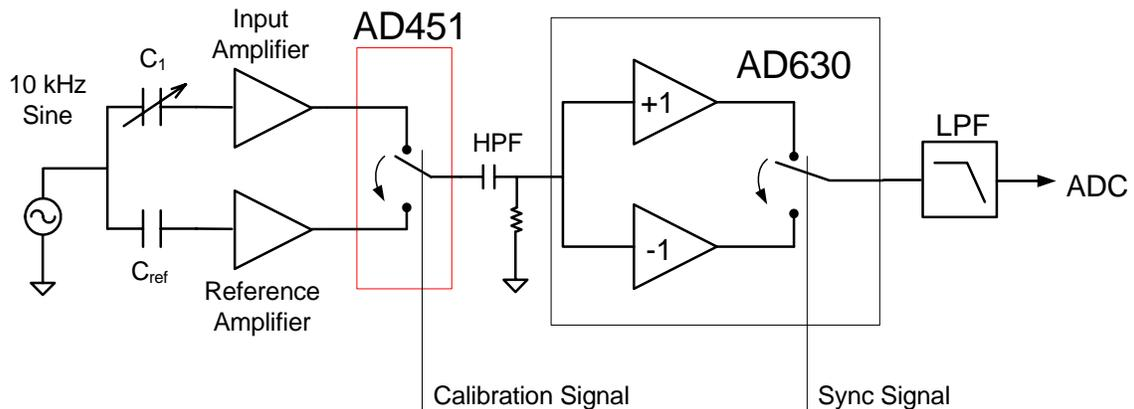
**Figure 16: Switched calibration circuit**
