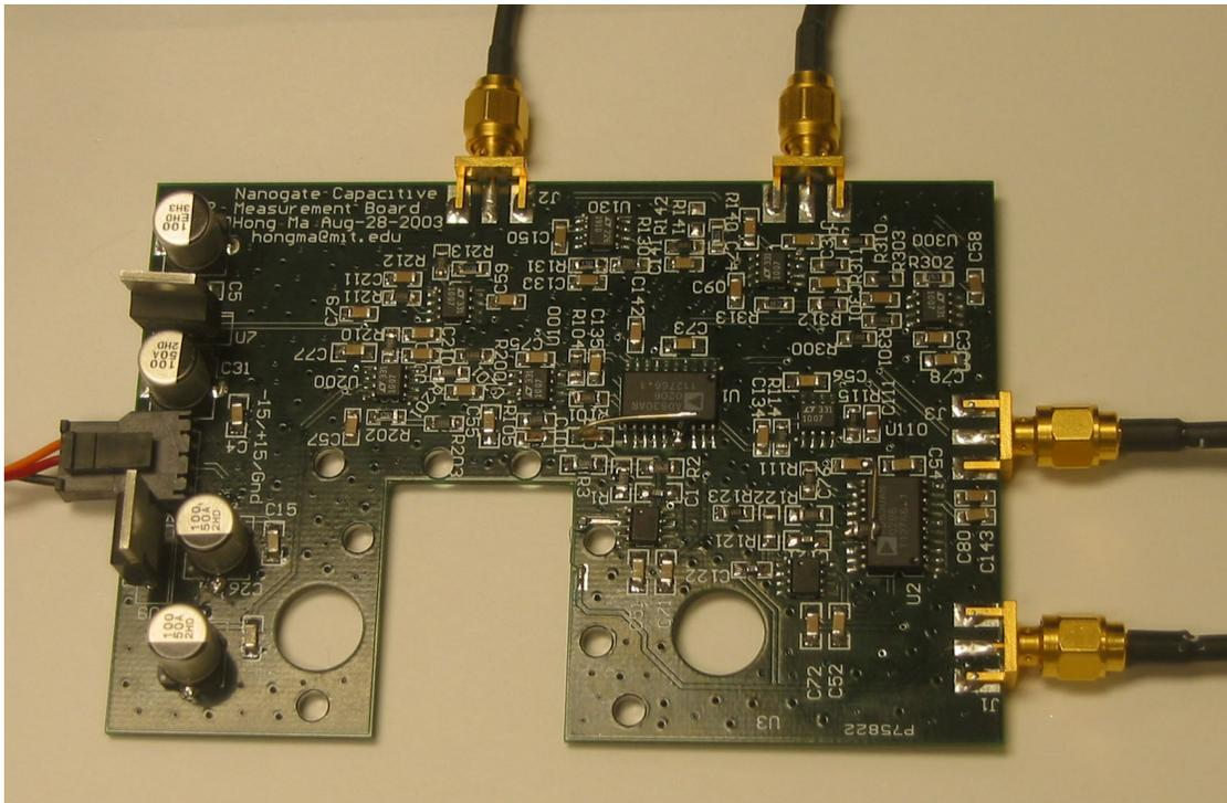
**Figure 20: Photograph of the analog front-end PCB**
