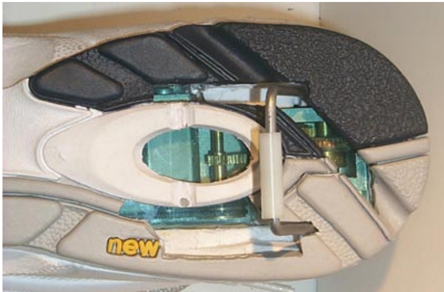
Figure 3.2 - Completed power generation in heel of shoe
