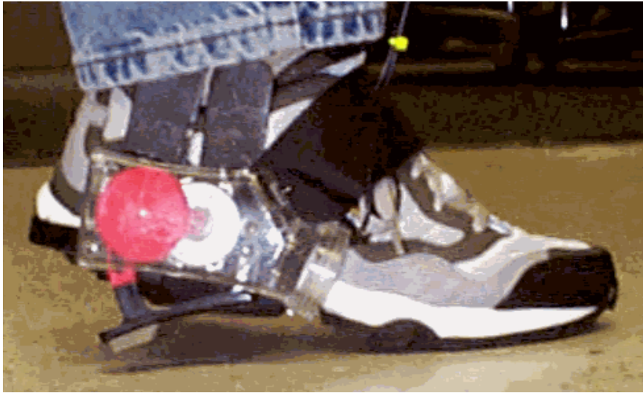
Figure 2.3: Picture of electromechanical generator attached to shoe during tests
