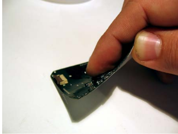
Figure 3-10: Node with electrical components being flexed
