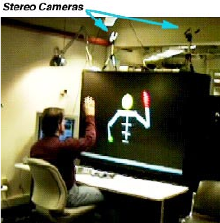
Figure 1-4: The Media Lab's SmartDesk, Tracking hands with Multiple Cameras
