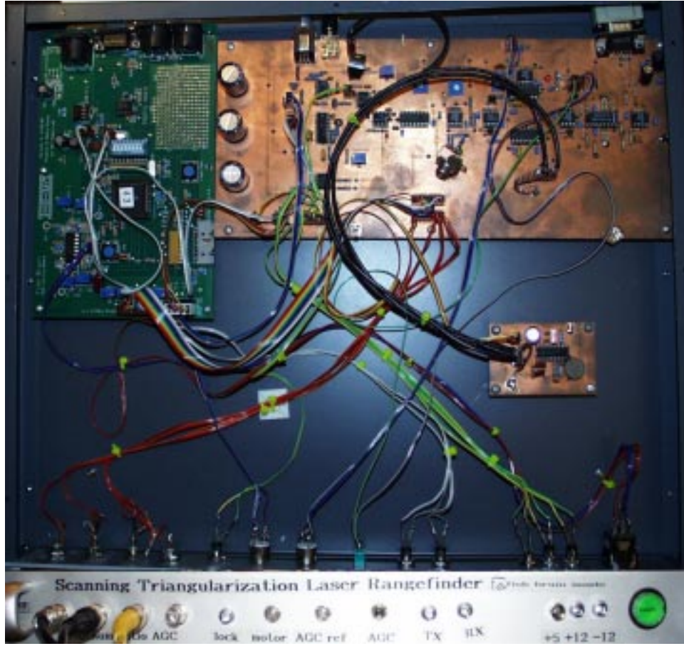
Figure 3-3: Triangulation Position Detection Circuitry
