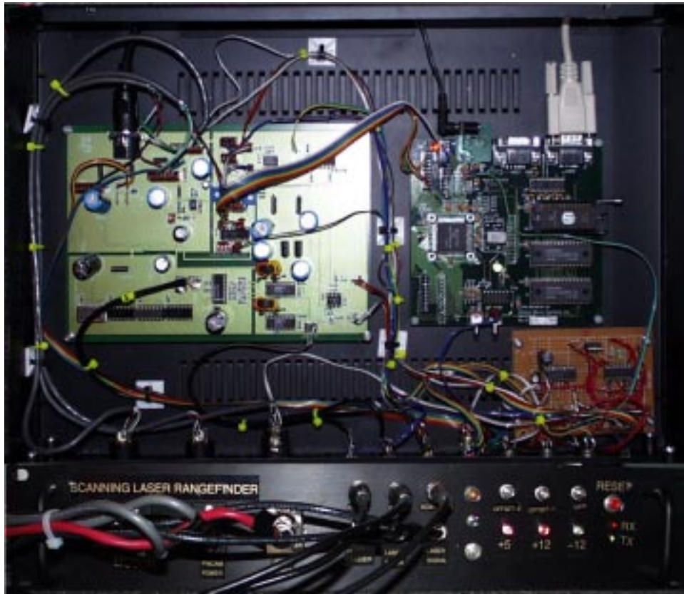
Figure 3-9: Demodulation Electronics Rack Unit
