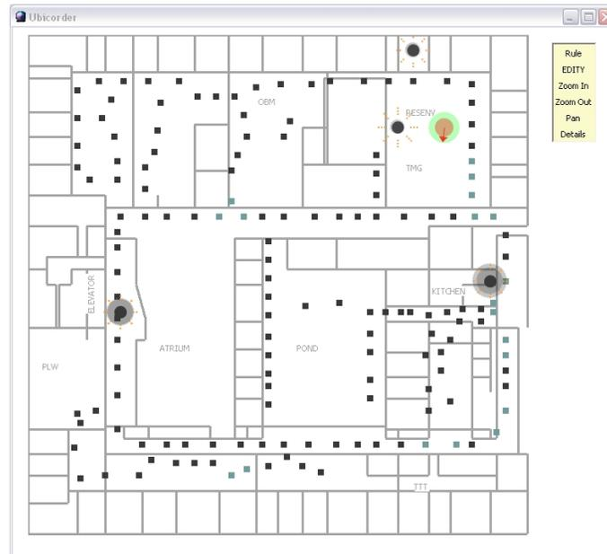
Figure 6-1: Test Setup: Location of nodes. One “Spinner” node was deployed next to the elevator, another in the kitchen. One node was deployed “Resenv” (Responsive Environments area) near the microscope/soldering station. Another node close the Resenv Area is located within the author’s office. The nodes in the public areas (elevator, kitchen), have large halo’s (indicative of high sound levels). The nodes deployed in the Resenv area report low sound levels.
