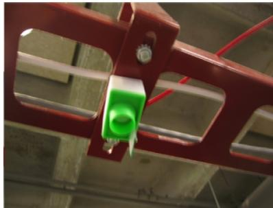
Figure 5-2: A “MERL” [31] movement node mounted on the ceiling
