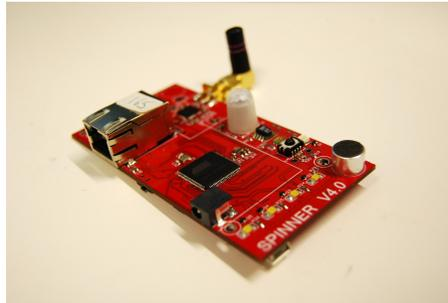
Figure 5-3: A “Spinner” sensor node, designed by Mathew Laibowitz
