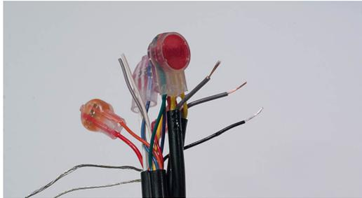
**(m)** Step 13. Strip the Ground Wires
