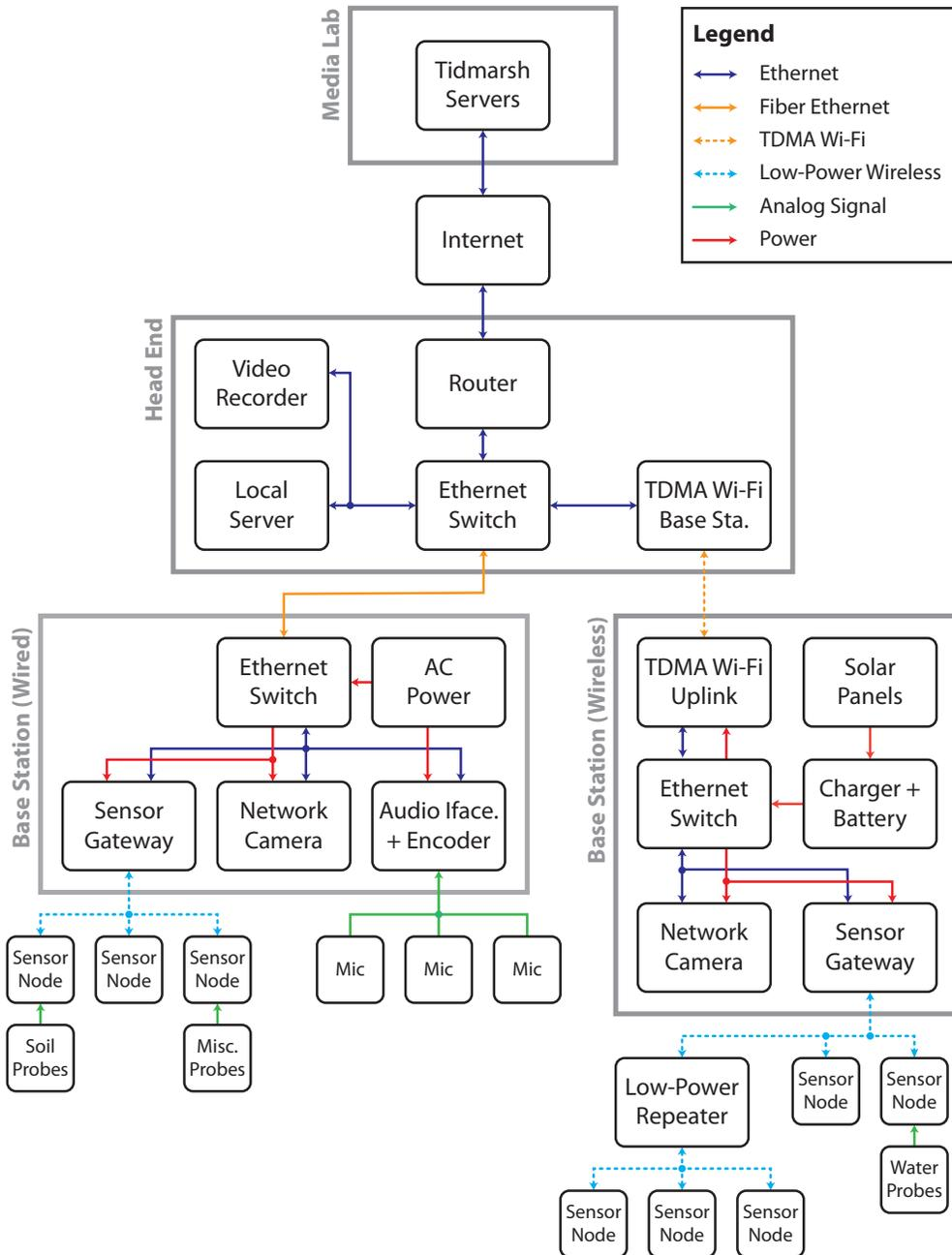
**Figure 3.1:** Schematic diagram showing the physical structure of the Tidmarsh sensor network as of the summer of 2020. Note that there are more base stations, sensor nodes, cameras, etc. than represented here.
