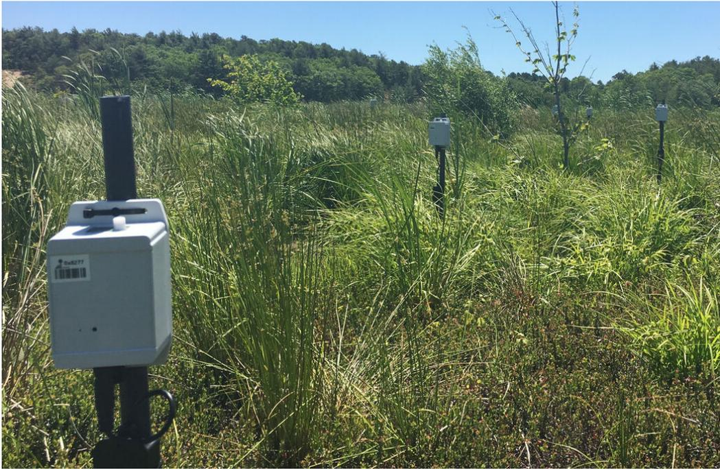
**Figure 3.11:** Second-generation nodes in the microtopography cluster.
