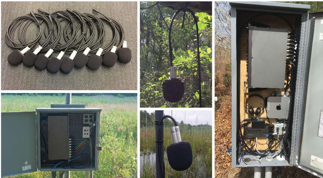
**Figure 4.4:** Audio installation at the Impoundment: microphones ready for deployment and in the field, main base station (right), satellite box (lower left).
