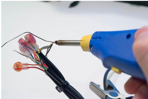
**(o)** Step 15. Solder the Ground Wires
