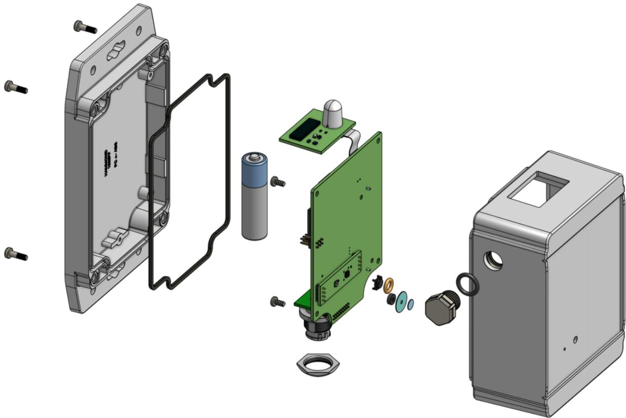
**Figure 3.6:** Second-generation sensor node assembly, exploded view
