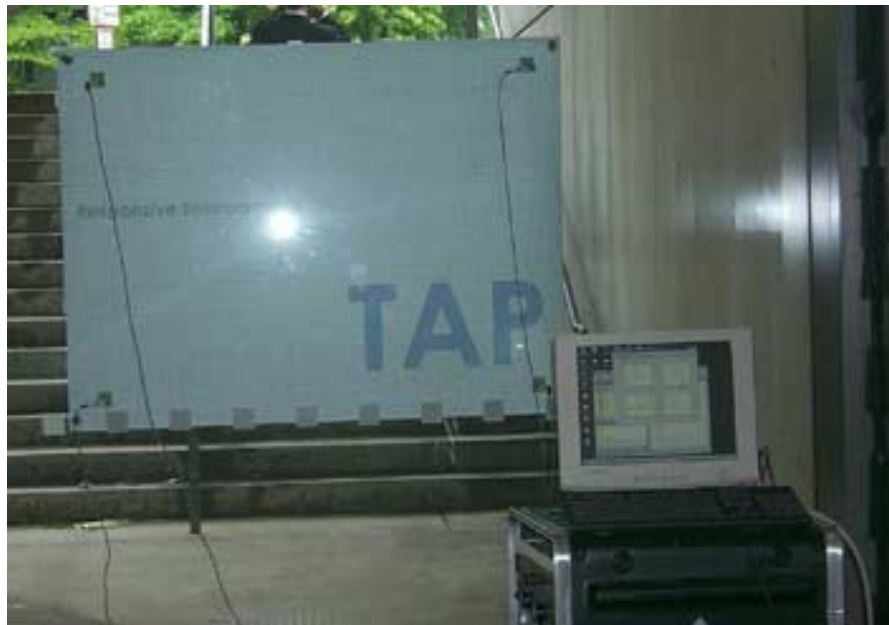
FIGURE 6-1: Picture of the acoustic tap tracker setup in the atrium of the MIT Media Lab. The effective area of enclosed by the sensors is approximately 35 inches by 47 inches. The computer was used for DAQ.
