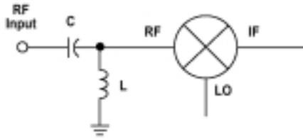
**Figure 44. HPF architecture used for matching the mixer's RF port.**
