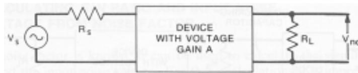
**Figure 23. Set-up for measuring single-frequency (spot) noise factors [34].**
