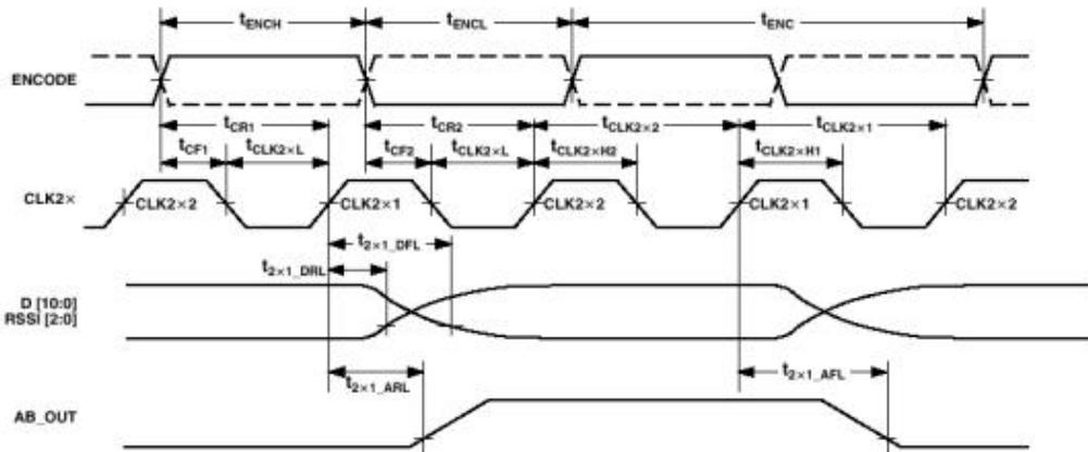
Figure 84. AD6600 timing diagram: encode to CLK2x delays and CLK2x propagation delays [72].
