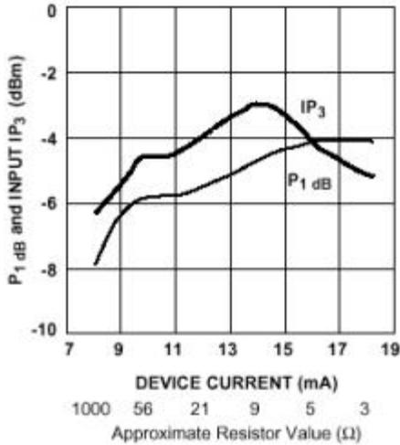
**Graph 10. Mixer's 1-dB compression point and IIP3 vs. device current (resistor value) [57].**
