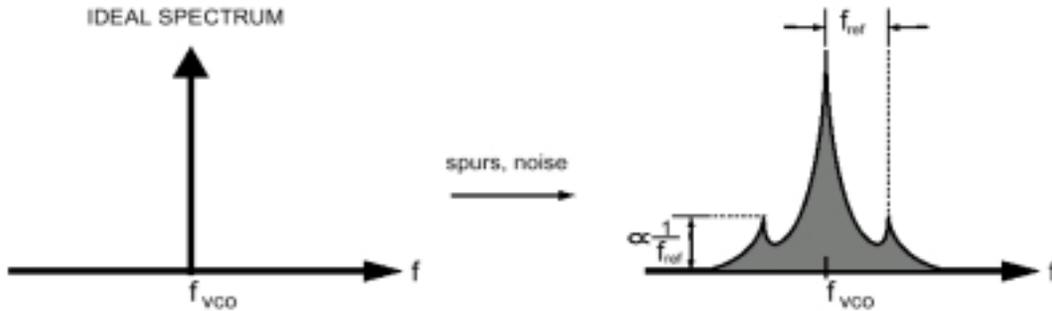
**Figure 54. Illustration of reference spurs [23].**
