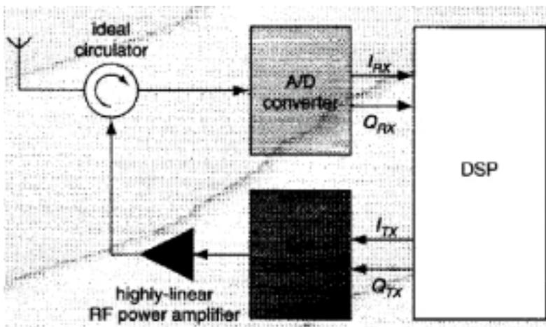
**Figure 7. “Ideal” SDR with transmitting and receiving capabilities [5].**
