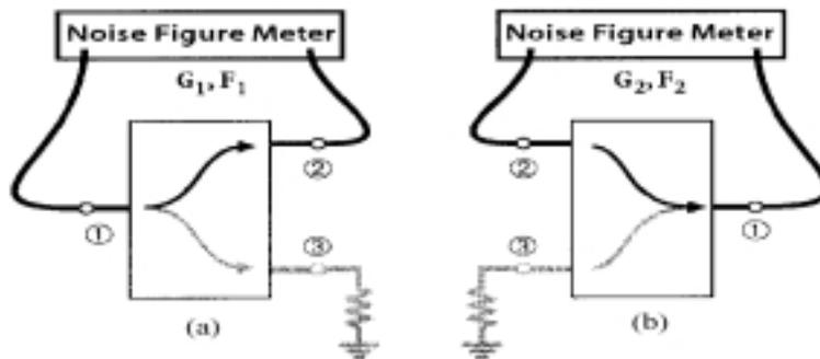
**Figure 26. Test set up for a two port measurement of noise figure and gain on (a) power-splitting balun and (b) power-combining balun [37].**
