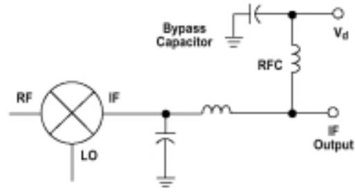
**Figure 45. LPF architecture used for matching the mixer's IF port. Mixer is DC biased through the IF port.**
