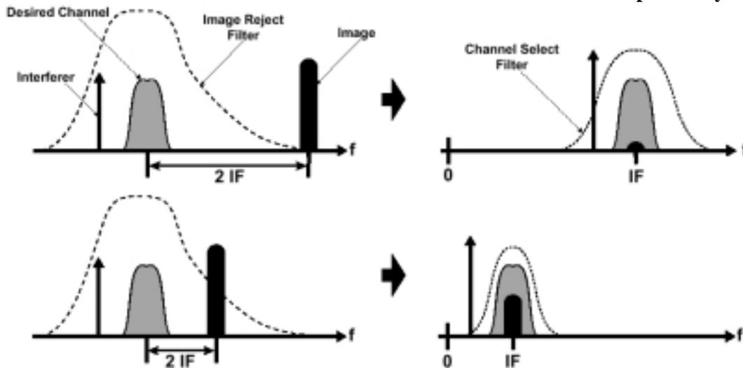
Figure 20. Importance of an image rejection filter before downconversion.
