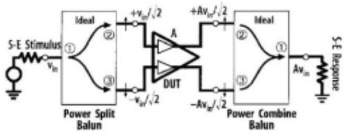
**Figure 25. Differential amplifier, with gain A, surrounded by two ideal baluns [37].**
