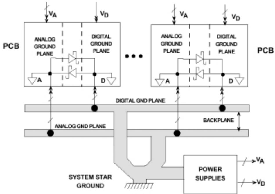
Figure 93. Using diodes to separate analog and digital ground planes.
