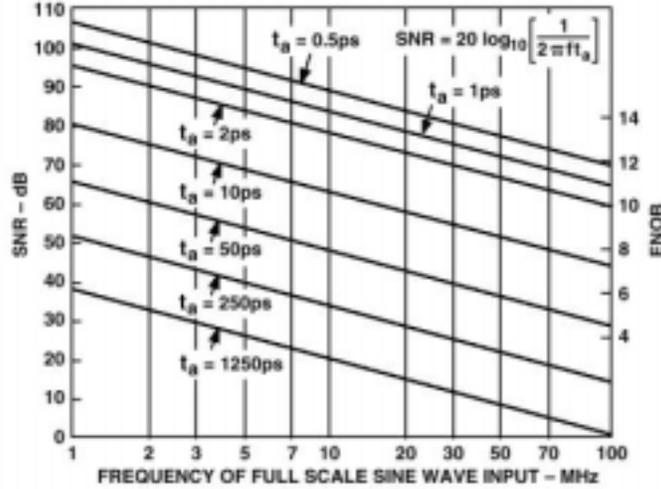
Graph 13. SNR due to aperture and sampling clock jitter [71].
