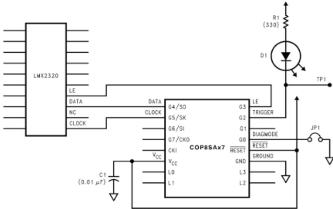
**Figure 56. Connections between the microcontroller and the frequency synthesizer [67].**
