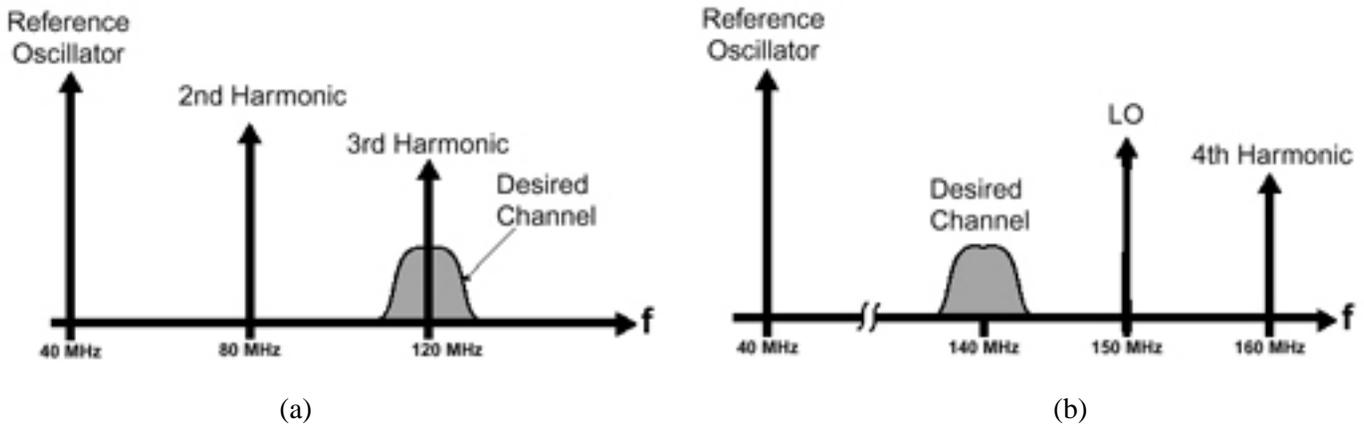
**Figure 12. Location of the IF determines if a reference oscillator’s harmonics cause in-channel signal degradation (a), or not (b) [23].**
