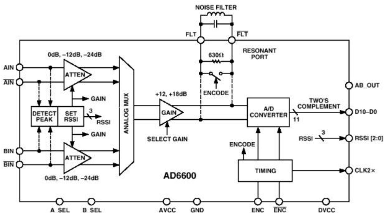
Figure 80. Functional block diagram of the ADC [72].
