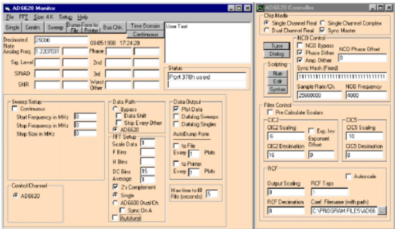
Figure 90. AD6620 evaluation board's control program [75].
