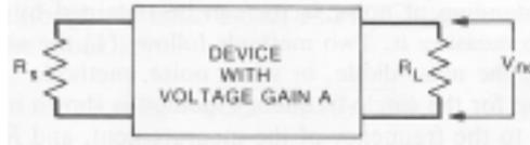
**Figure 22. Resistive source used for noise factor measurements[34].**
