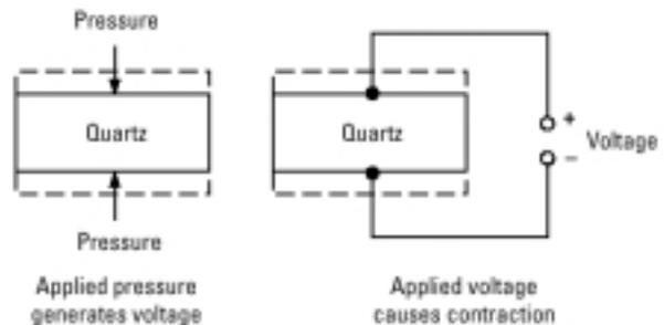
**Figure 63. Piezoelectric properties of crystal [68].**
