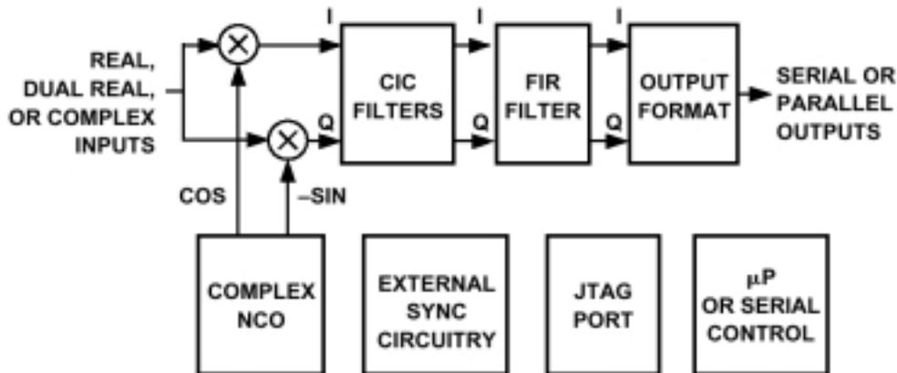
**Figure 88. Functional block diagram of the AD6620, with four cascaded signal processing elements: a frequency translator, two fixed coefficient decimating filters, and a programmable coefficient decimating filter [76].**
