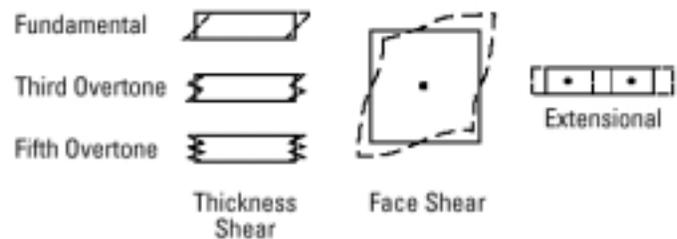
**Figure 65. Crystal cut and thickness shear determine vibration modes [68].**
