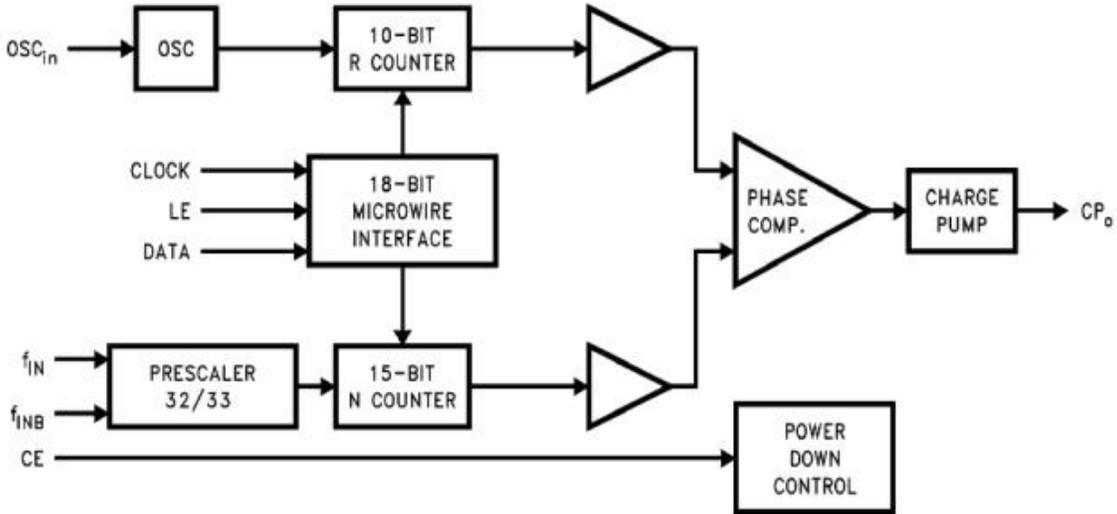
Figure 51. LMX2324 2.0 GHz Frequency synthesizer’s block diagram [60].
