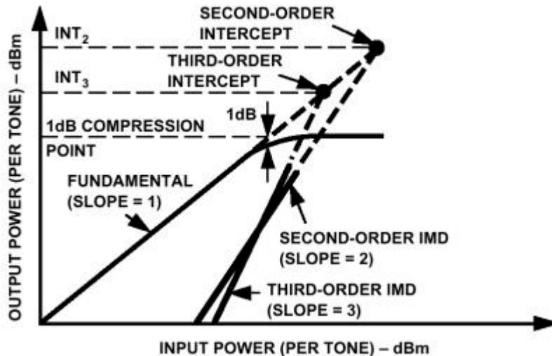
**Figure 30. Intercept points, gain compression, IMD [21, pg 25]**
