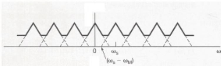
**Graph 4. Frequency plot illustrating sampled signal with aliasing [15].**
