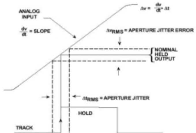
**Figure 76. The effects of aperture and sampling clock jitter [8, see pg. 4-28].**
