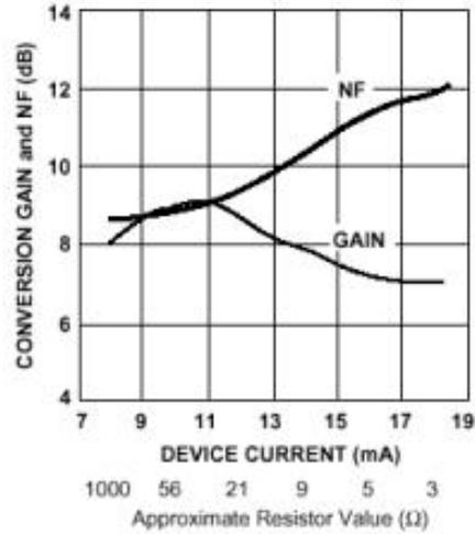
**Graph 11. Conversion gain and noise floor vs. device current (resistor value) [57].**
