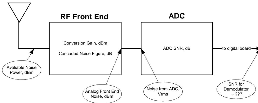
Figure 21. Sensitivity measurement calculation.
