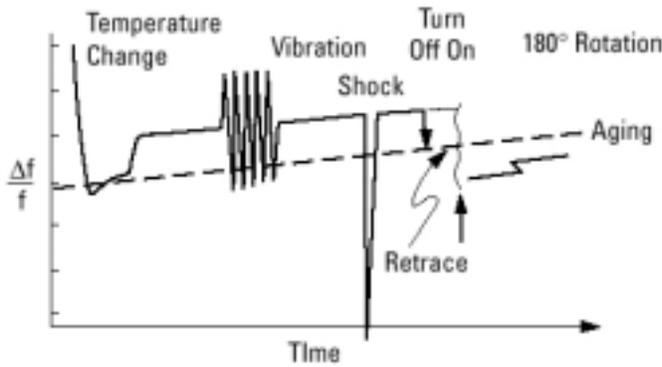
**Figure 73. Environmental effects on fractional frequency stability.**
