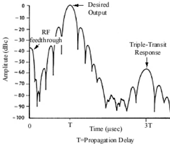
Graph 9. Impulse response of a typical SAW filter[27].
