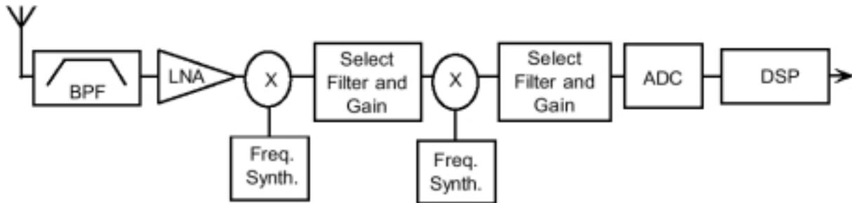
Figure 4. Typical single-carrier receiver [9]
