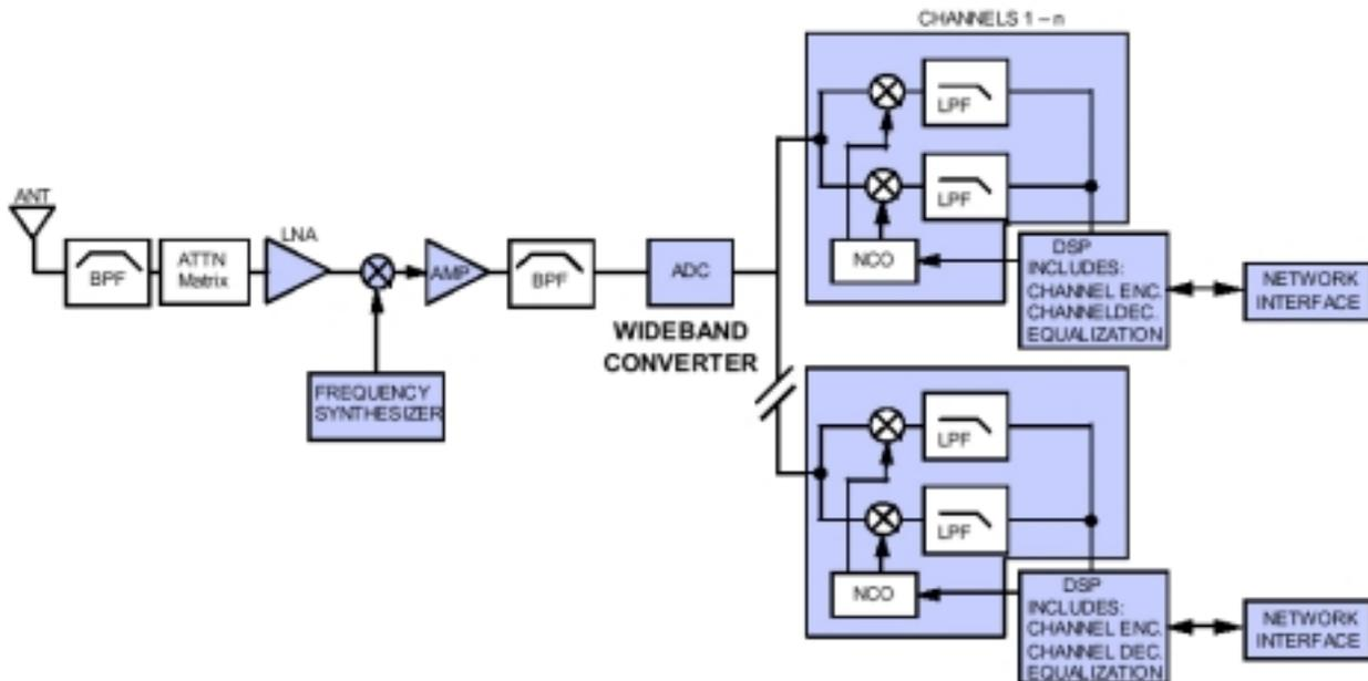
Figure 5. Typical multi-carrier receiver [9]
