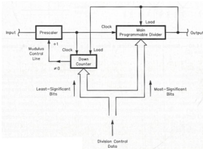
Figure 52. Functional block diagram of a dual-modulus prescaler [17, pg 14.37].
