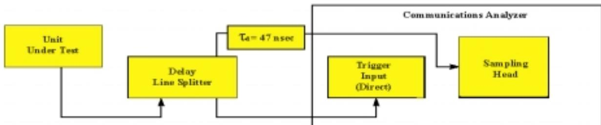
**Figure 74. Using a delay line and a communications analyzer to locate the reference edge and examine the jitter on subsequent clock edges [1].**
