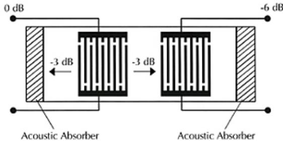
**Figure 59. Simple transversal SAW filter configuration [27].**
