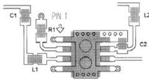
**Figure 39. Recommended PCB layout for the LNA, [53].**
