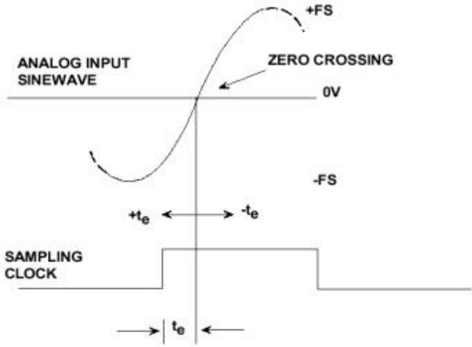
Figure 3. Jitter is when the sampling clock edge's location changes over time [8, see pg 4-29].
