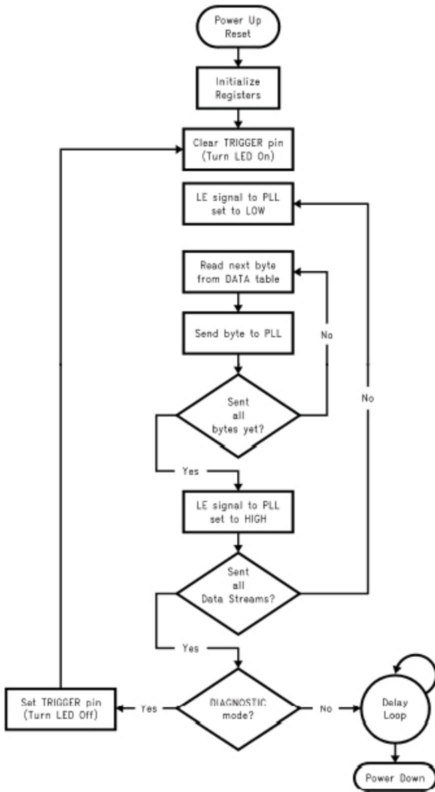
Figure 58. Flow chart illustrating connection between the microcontroller and the frequency synthesizer [67].
