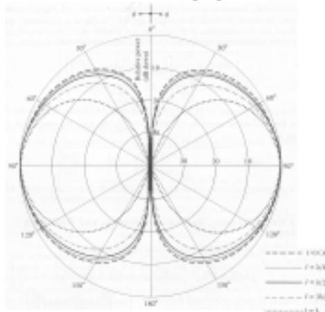
**Figure 36. Radiation pattern of an antenna depends on its length [44].**
