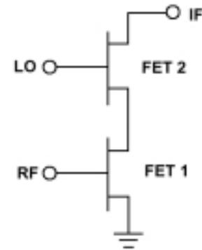
**Figure 41. Cascode-connected pair of FETs make the mixer.**
