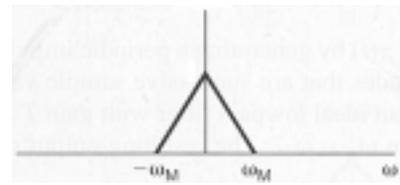
**Graph 1. Frequency representation of a band limited signal that will be sampled in the time domain [15]**
