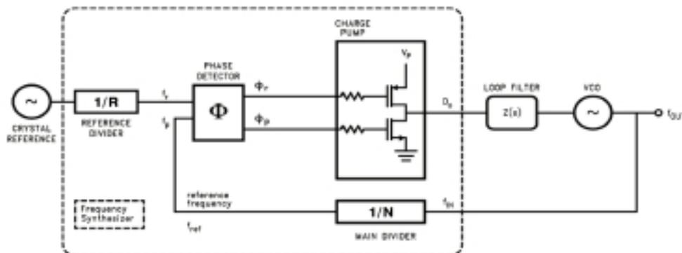
Figure 47. Basic charge pump PLL [59, pg 18].
