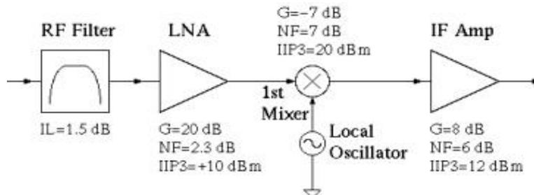
**Figure 28. Block diagram with typical gain, noise figure, third intercept points information.**
