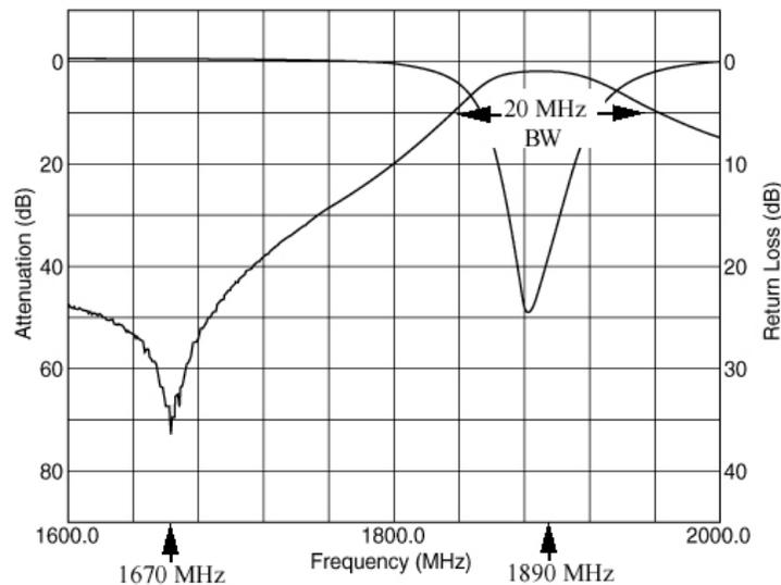
**Figure 38. BPF’s pass band is 20 MHz wide and maximum attenuation at 1.670 GHz [see 52].**
