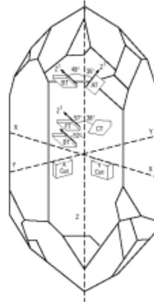
**Figure 66. Doubly terminated quartz crystal's typical axis cuts [68].**
