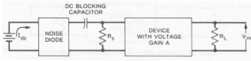
**Figure 24. Noise-diode method of measuring integrated noise factors, i.e. white noise[34].**
