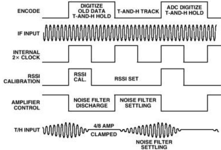
Figure 83. AD6600: ADC's internal timing [72].
