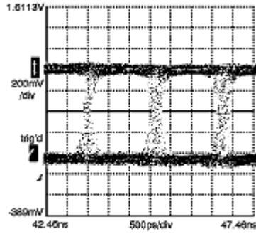
**Figure 78. Effects of medium amounts of jitter [69].**
