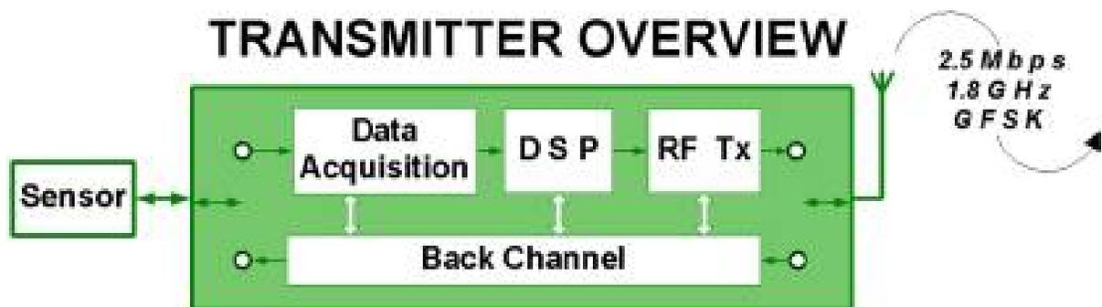
Figure 13. Transmitter block diagram.
