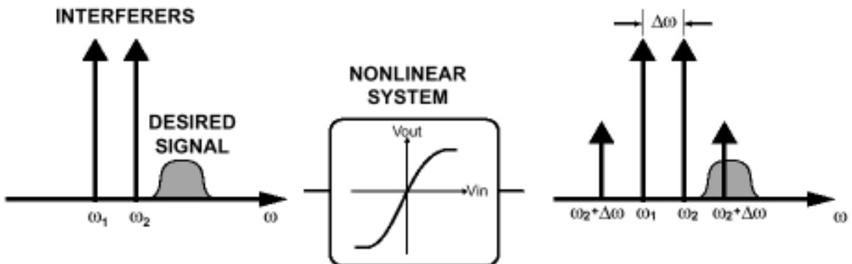
**Figure 11. Illustration of nonlinear system producing undesirable intermodulation products that lie in the desired signal's passband.**
