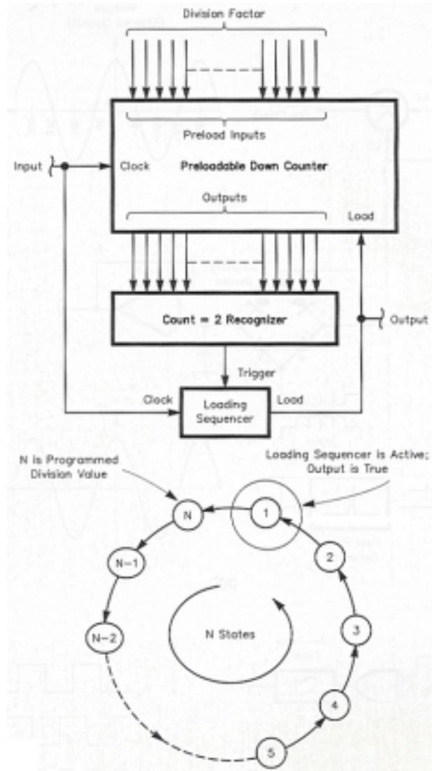
**Figure 48. The mechanism of a frequency synthesizer [17, pg 14.37].**
