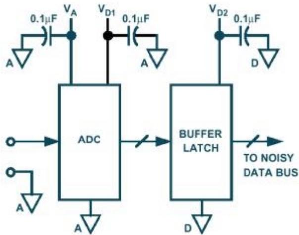
Figure 95. Buffering the outputs of the ADC to reduce noise on ADC inputs [87, pg 21].
