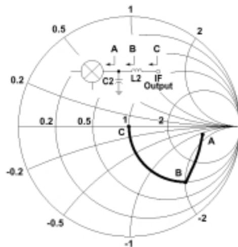
**Figure 43. Smith chart used to impedance match the mixer's IF port [57].**
