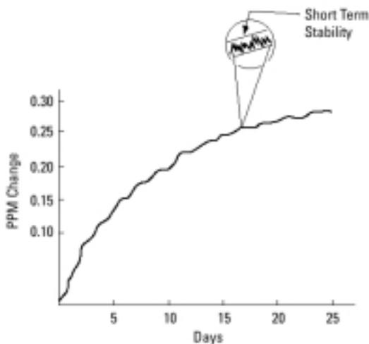
**Figure 71. Long term (ppm) and short term (jitter) fractional frequency stability [68].**
