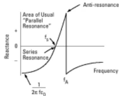
**Figure 68. How a crystal's reactance varies with frequency [68].**
