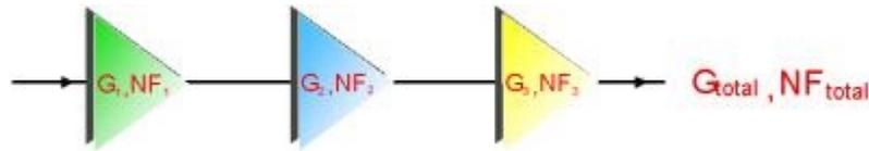
**Figure 27. Block diagram of cascaded noise figure [39].**
