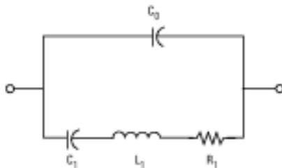
**Figure 67. Electrical model for quartz resonator [68].**
