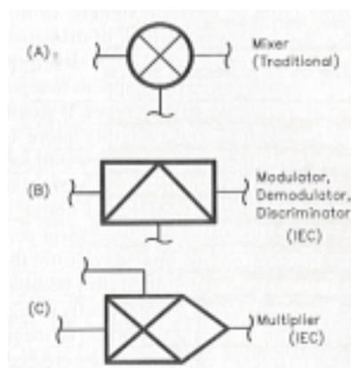
**Figure 40. Three types of signal multipliers [17].**
