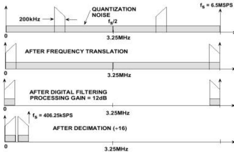
Figure 82. digital filtering and decimation example [74, see pg 5-29].
