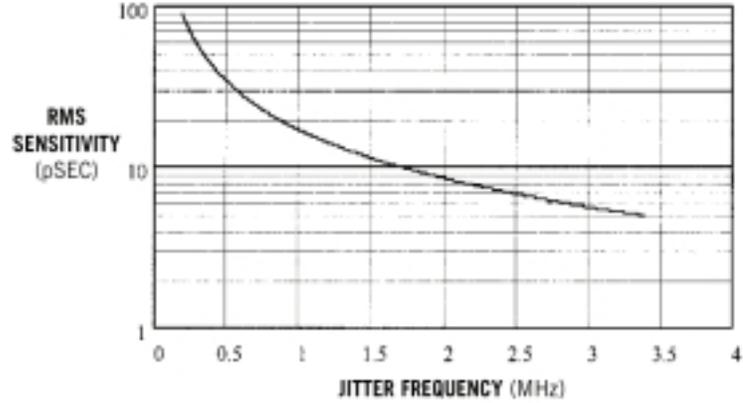
**Graph 12. 47 nsec delay line jitter sensitivity [1].**
