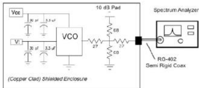
Figure 97. Phase noise measurement set-up of the VCO [89].
