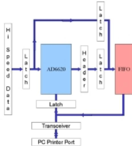
**Figure 87. Block diagram of the AD6620 evaluation board [75].**
