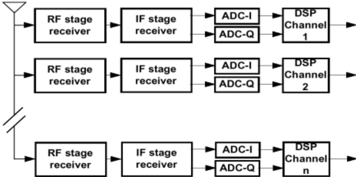
**Figure 6. Narrowband architecture used in a base station receiving multiple channels [10]**
