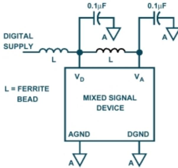
Figure 92. Use of ferrite beads to isolate power planes [87].
