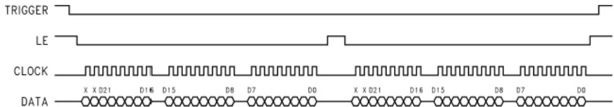
**Figure 57. Timing diagram of programming the frequency synthesizer on system start-up [67].**
