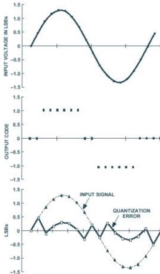
Graph 14. An illustration of quantization noise and square waves and dithering [73].
