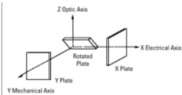
**Figure 64. Choice of axis and angles to cut crystal [68].**
