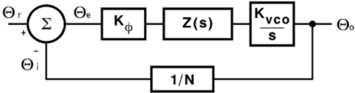
**Figure 53. Linear mathematical model of a PLL [59].**
