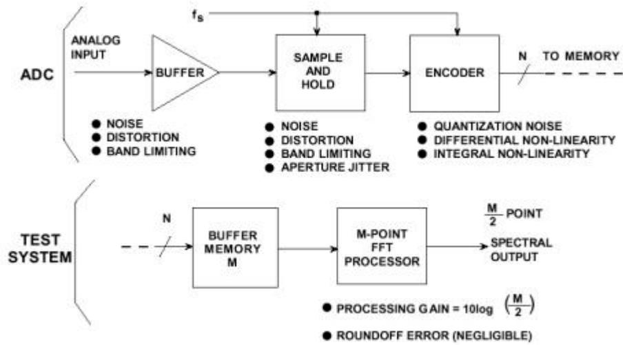
Figure 81. ADC model showing noise and distortion sources [8, see pg 4-14].
