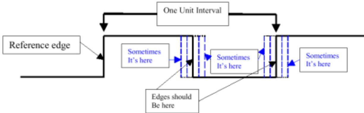
**Figure 62. Digital waveform with jittered edges [69].**
