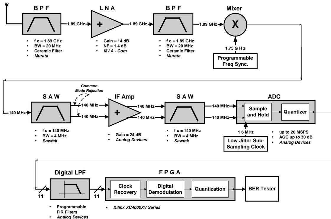
Figure 15. Detailed block diagram of base station.
