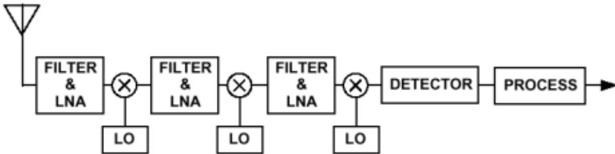
Figure 9. Typical receiver Block diagram [14].
