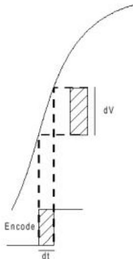
**Figure 75. Diagram to help understand aperture uncertainty calculation [9].**
