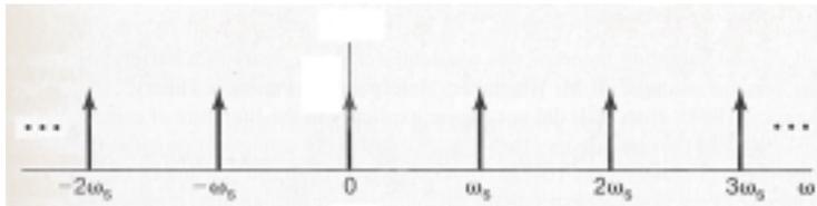
**Graph 2. Sampling in time translates to convolution with an infinite-impulse train in frequency [15].**
