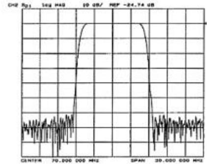
Figure 19. SAW frequency response with optimal layout [27].
