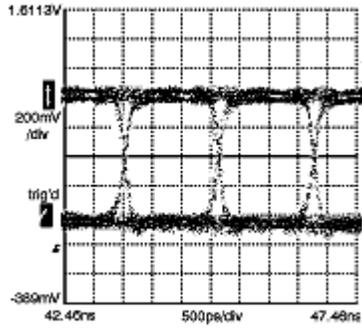
**Figure 77. Eye diagram with no jitter [69].**
