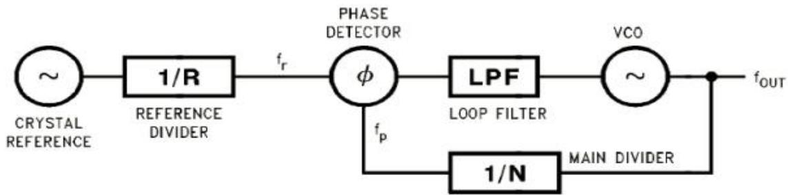
(a) Block diagram of a basic PLL.
