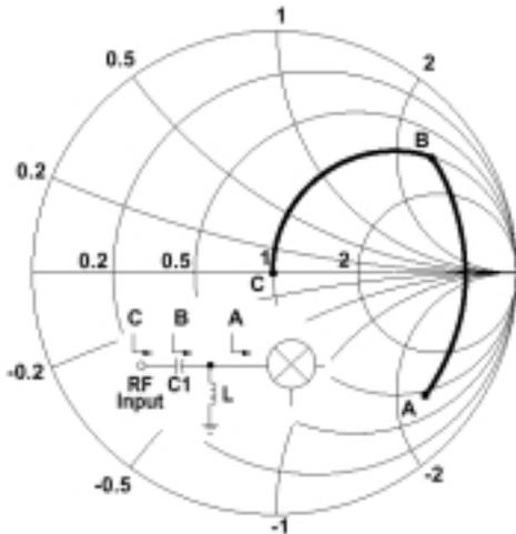
**Figure 42. Smith chart used to impedance match the mixer's RF port [57].**
