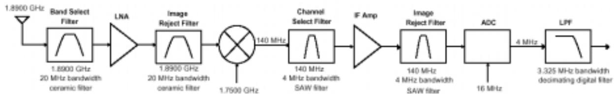
Figure 16. Frequency plans for the RF front end.
