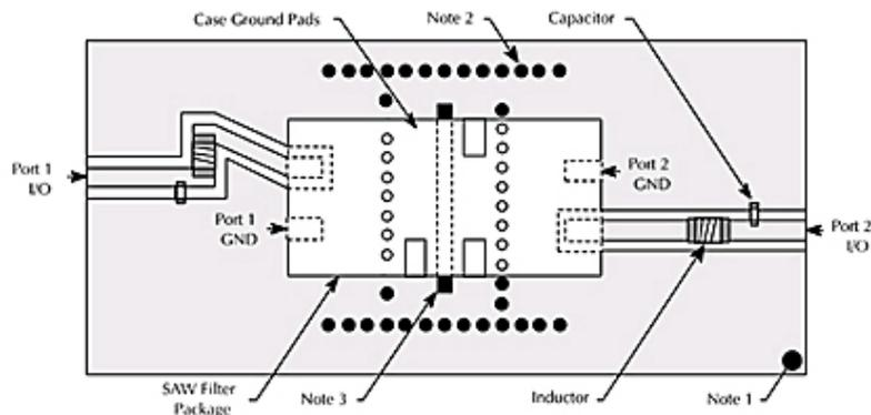
**Figure 61. Optimal PCB layout for SAW filter [27].**
