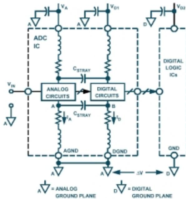
Figure 94. Grounding an ADC's digital pin on AGND plane [87].
