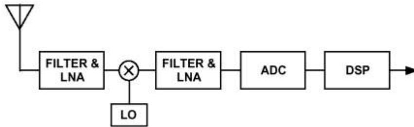
Figure 8. Digital receiver block diagram [14].
