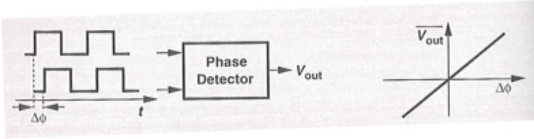
**Figure 49. Illustration of an ideal phase detector [43, pg 250].**
