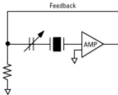
**Figure 70. Simple oscillator feedback circuit using a quartz resonator [68].**
