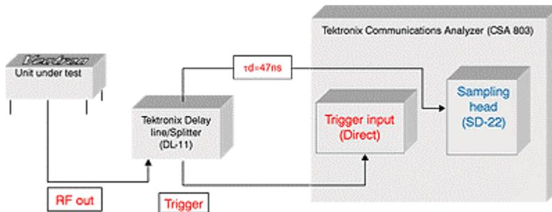
Figure 96. Testing setup recommended to measure jitter over time [69].
