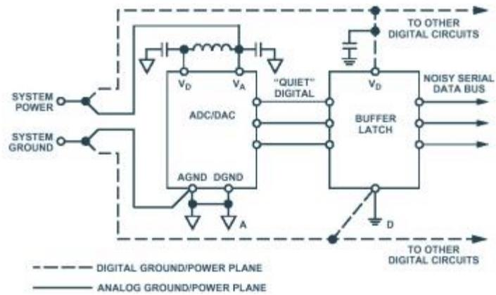
Figure 91. Separating the analog and digital grounds [86].
