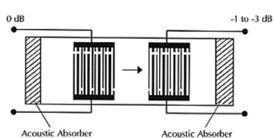
**Figure 60. Single-phase unidirectional filter configuration [27].**
