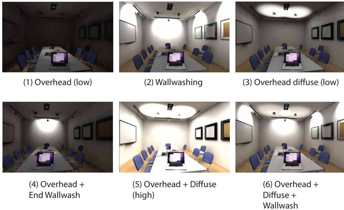
Figure 4.2: The six lighting scenes evaluated in the study (after Flynn et al., 1973).
