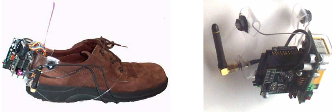
Figure 4-2: Wearable gait analysis platform and sensor attachment
