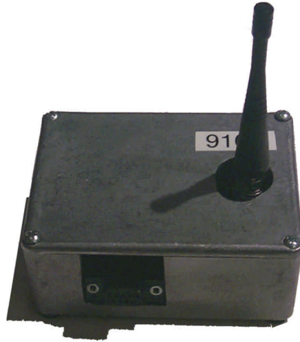
Figure 2-5: Current Basestation in Shielded Case
