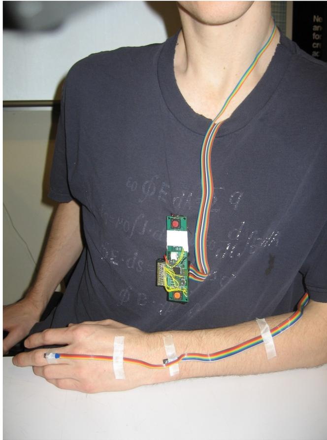
Figure A.1: Sensor System as Worn by User
