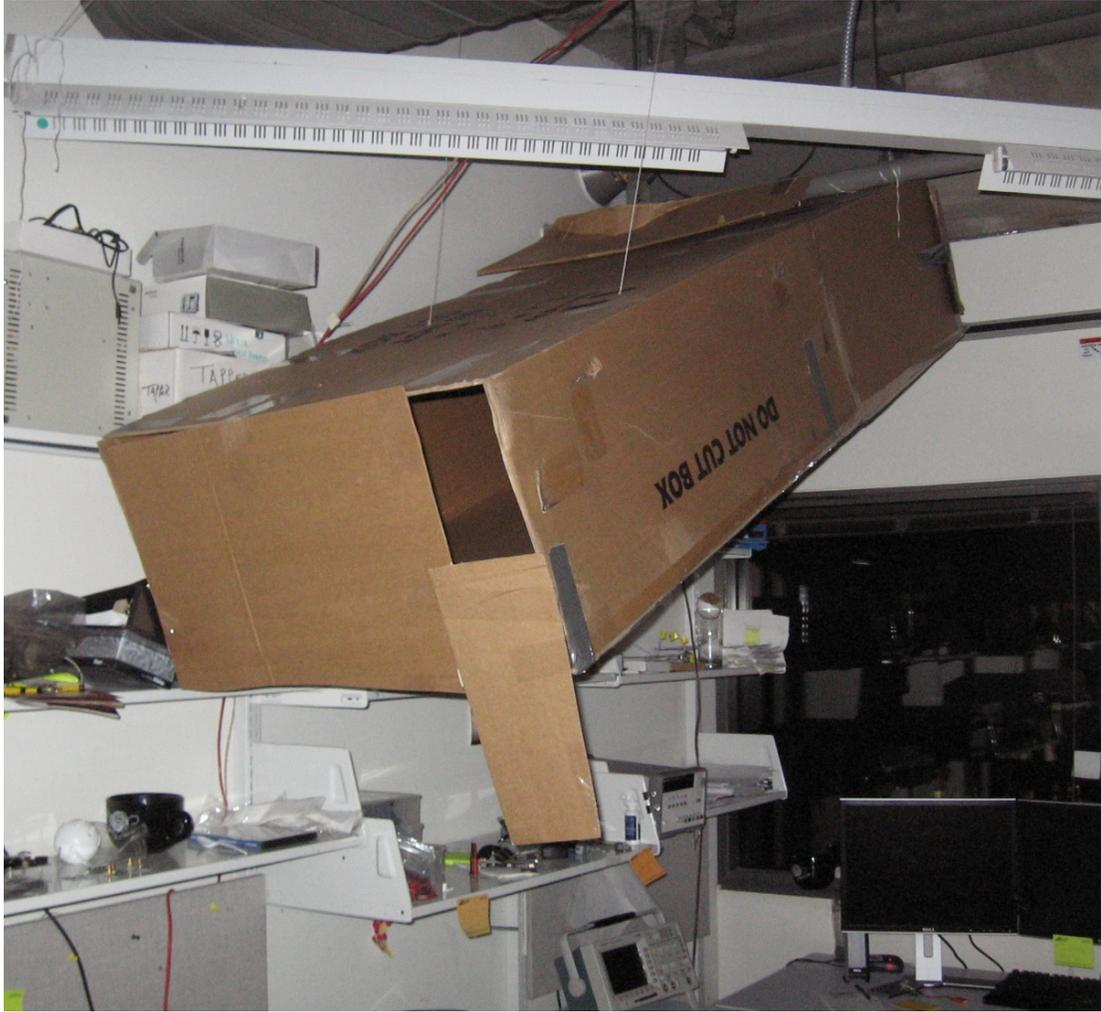
Figure 3.4.5: Collimator for In-situ Wind Speed Sensor Test
