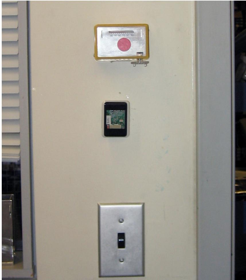
Figure 3.3.5: Portable Node Mounted Near Thermostat
