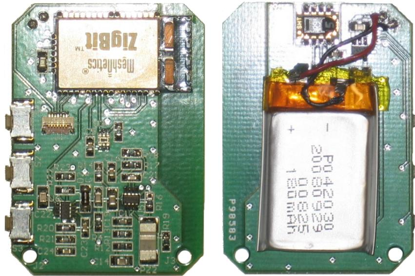
Figure 3.3.1: Portable Node Circuit Boards: Front and Back
