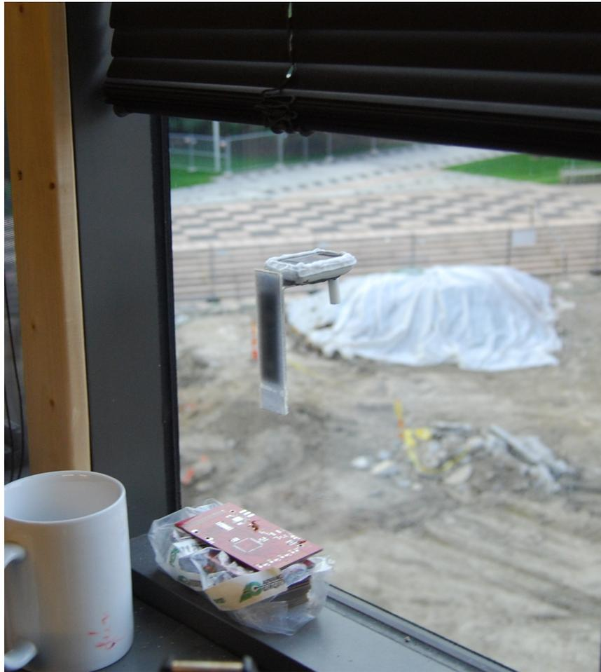
Figure 3.3.6: Portable Node Mounted on Exterior of Building
