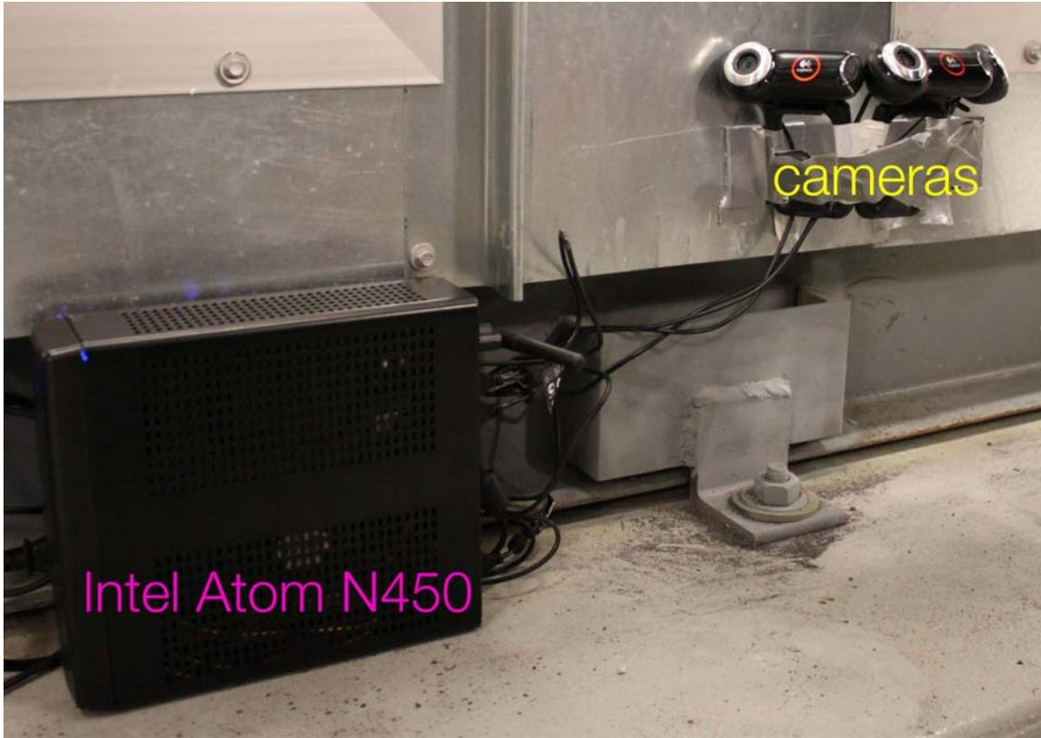
Figure 8: Low-power computer performs NTP time synchronization, bridges ZigBee network to the Internet using WiFi, and manages camera/vision subsystem.
