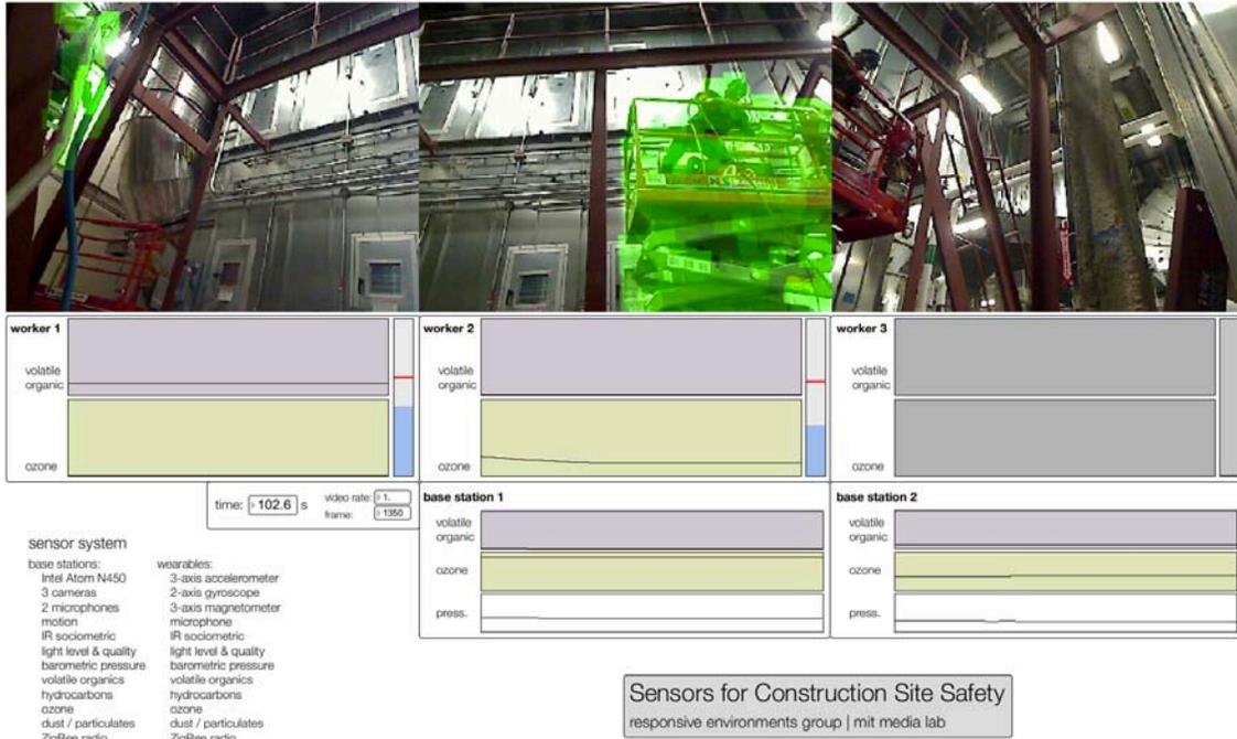
Figure 14: First version of the worker safety interface, showing un stitched video and altitude thresholds on each worker; when a worker passes the threshold set on the pressure sensor, the corresponding blob is marked in red.
