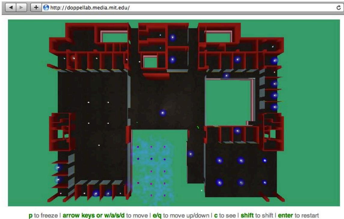
Figure 27: Top-view (floor plan view) in Doppellab. Also shown: application is embedded in a web browser, with identical functionality. In the web-based view, HTML instructions below the window change depending on user context, communicating with the application through JavaScript.
