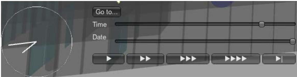
Figure 28: Interface for exploring historical sensor data; the top slider controls the time over a 24 hour period, and the bottom slider sets the date, going back as far as data is available. The buttons set the rate of playback, and the clock reflects the current simulation time and rate.
