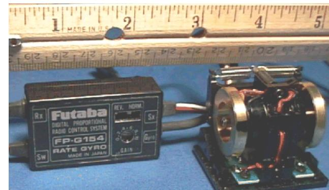
**FIGURE 1-2** Futaba FP-G154 Single Axis Gyroscope (Circa 1990)
