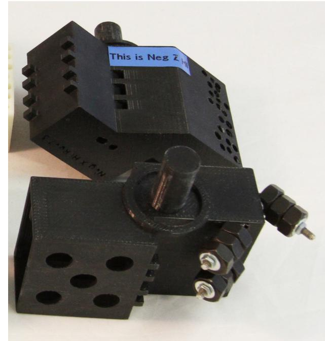
FIGURE 4-33 Hand Balanced Brackets. Removal of mass via drilling holes (Upper Bracket). Addition of mass by placing nuts on threaded screws (Lower Bracket).
