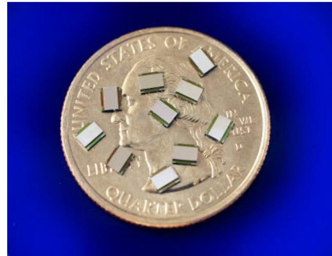
**FIGURE 1-1** Invensense IMU-3000 3-Axis Gyroscopes (2012)
