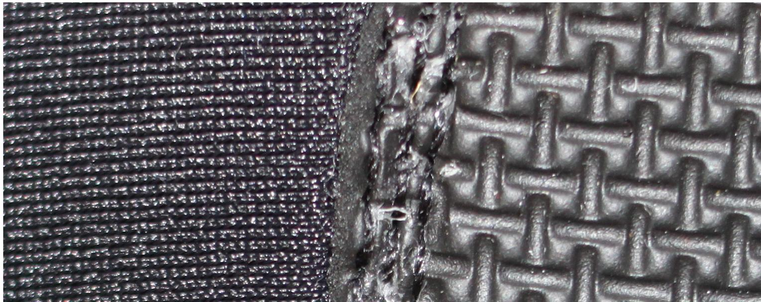
In order to secure the nodes, sleeves and straps into place on body segments, hook velcro was sewn into place.
