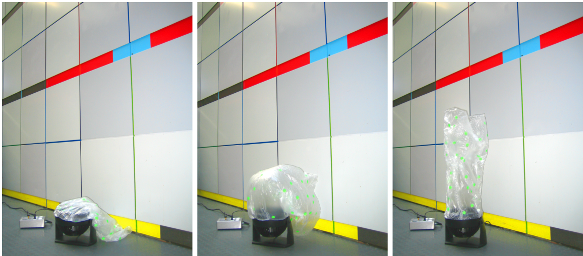
Figure 4-11: The real-world version of the data pond can display information according to how much air flow passes through the plastic shroud, which is controlled at a fine level of detail by the Plug used to power the data pond's fan.
