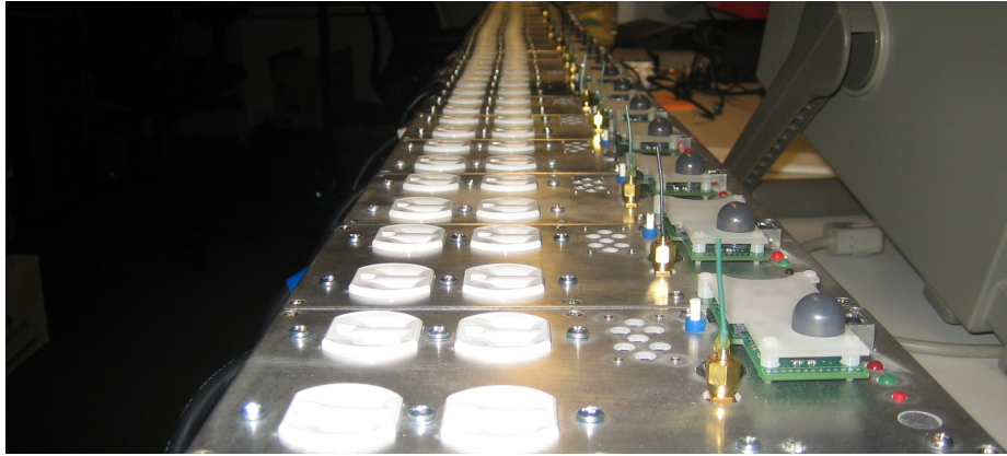
Figure 4-2: Plug sensor nodes in preparation for being programmed.
