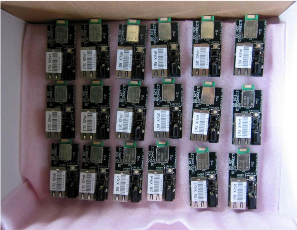
**Figure 4-7: Bluetooth Location beacons ready to be deployed**
