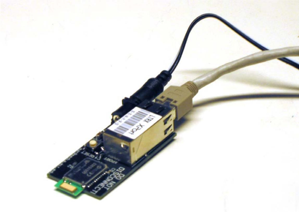
**Figure 4-8: Bluetooth beacon with LAN cable attached and power supply plugged in**
