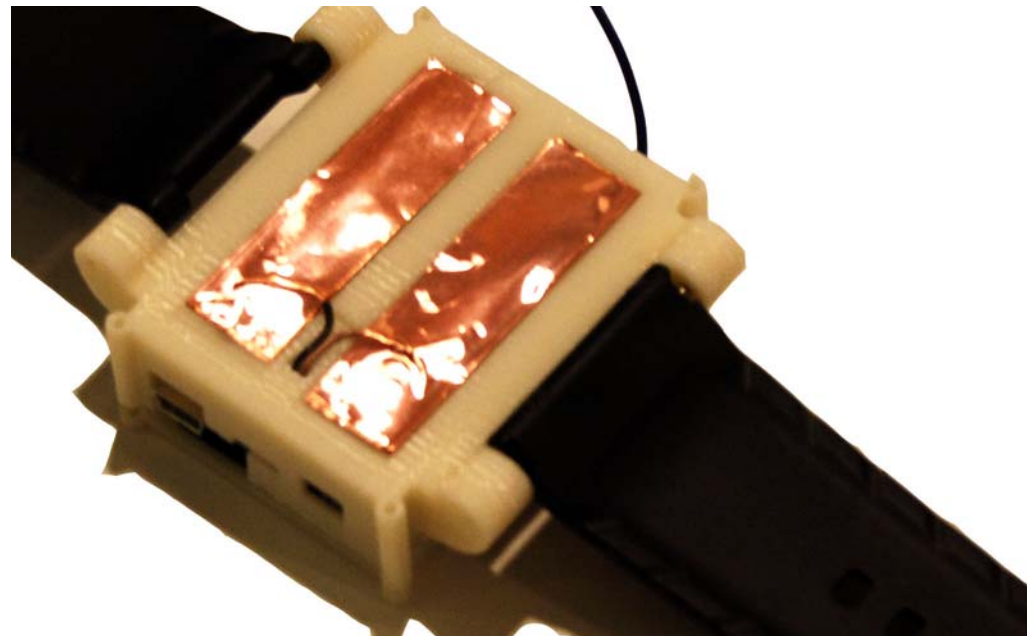
FIGURE 3-36 Wrist unit's GSR probes on arm side of device
