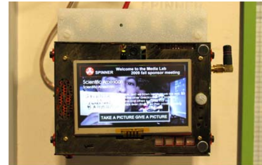
12 SPINNER node running the multipoint image capture and broadcast application
