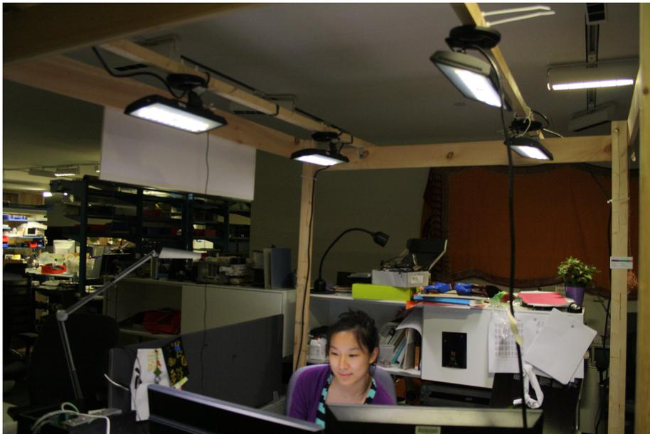
**Figure 3.1:** Commercial solid state lighting testbed
