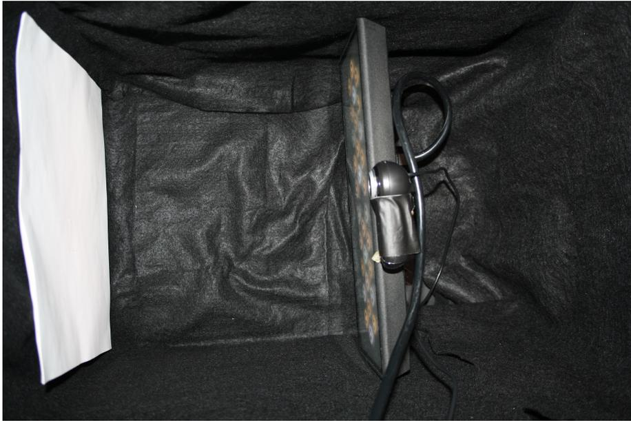
**Figure 3.15:** Webcam offline calibration setup
