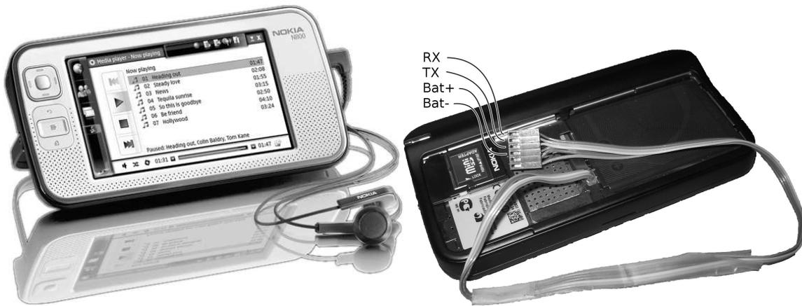
Figure 4-1: Front and back of N800, with serial port exposed in open back showing our custom adapter
