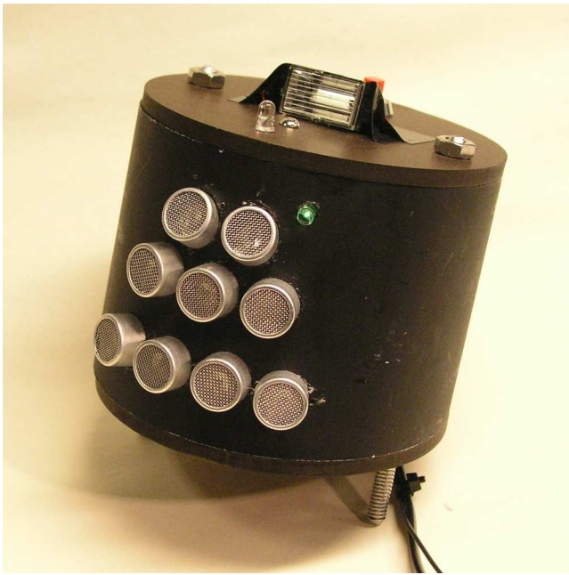
Fig. 4. The “pinger” delivers a simultaneous flash of light and burst of 40-kHz ultrasound. Each Pushpin can measure the difference in time of arrival of these two signals and use this to calculate the distance between itself and the Pinger.
