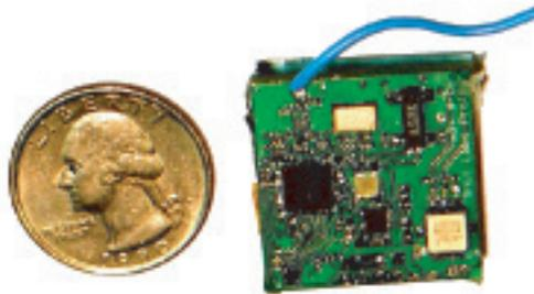
Figure 3.4: Early prototype of an narrative sensor node.
