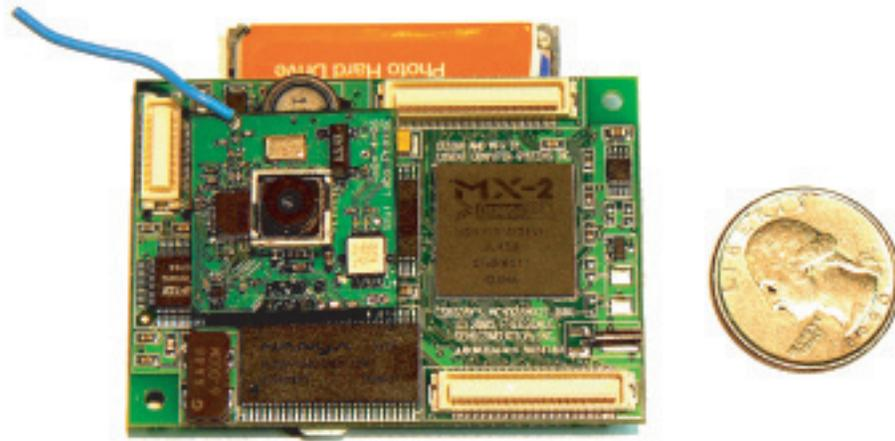
Figure 3.3: Early prototype of an imaging sensor node.
